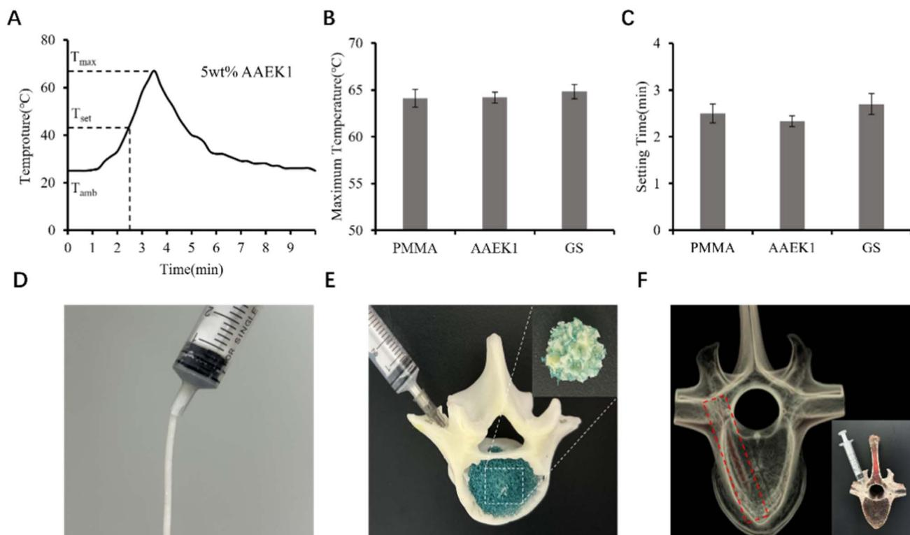
Fig. 6 Polymerization temperature, setting time, and operability of cement. (A) Polymerization temperature curve over time for 5 wt% AAEK1 cement. (B and C) Maximum polymerization temperature and setting time of PMMA, AAEK1 and GS cements. (D) Injectability of AAEK1 cement. (E) Evaluation of the filling and diffusion properties of AAEK1 cement in a 3D-printed human vertebral body model. (F) X-ray image after injection of AAEK1 cement.
