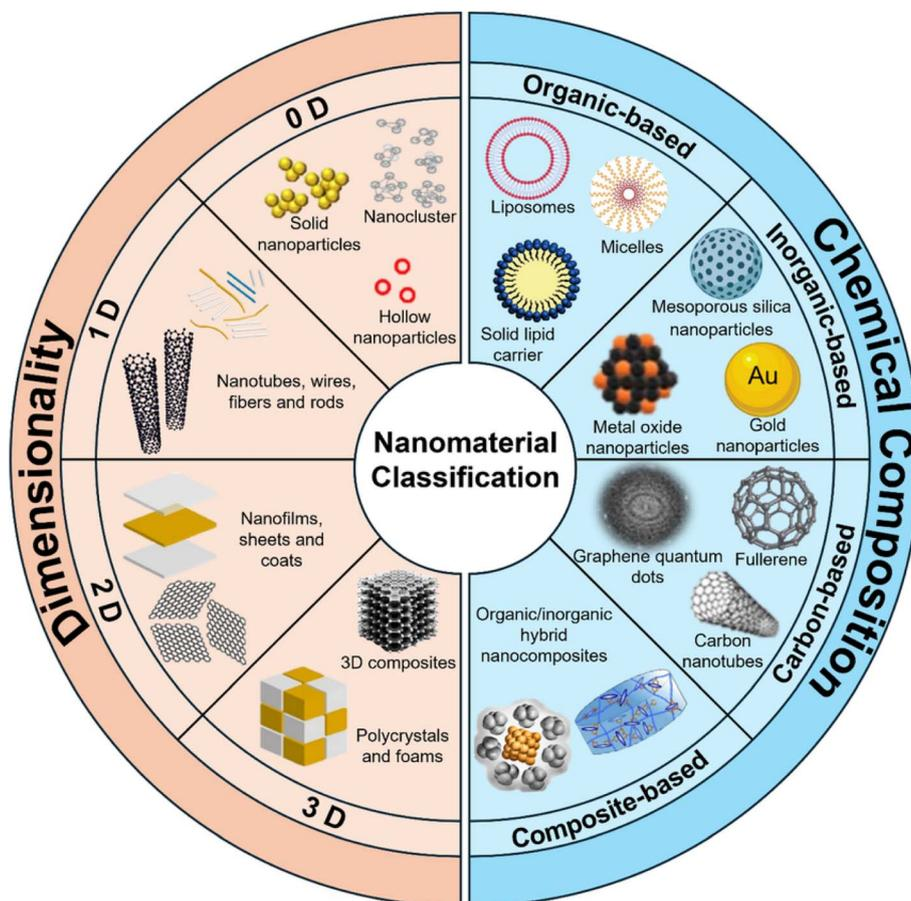
Fig. 2 Classification of nanomaterials used in biosensors for healthcare application.<sup>40</sup>
