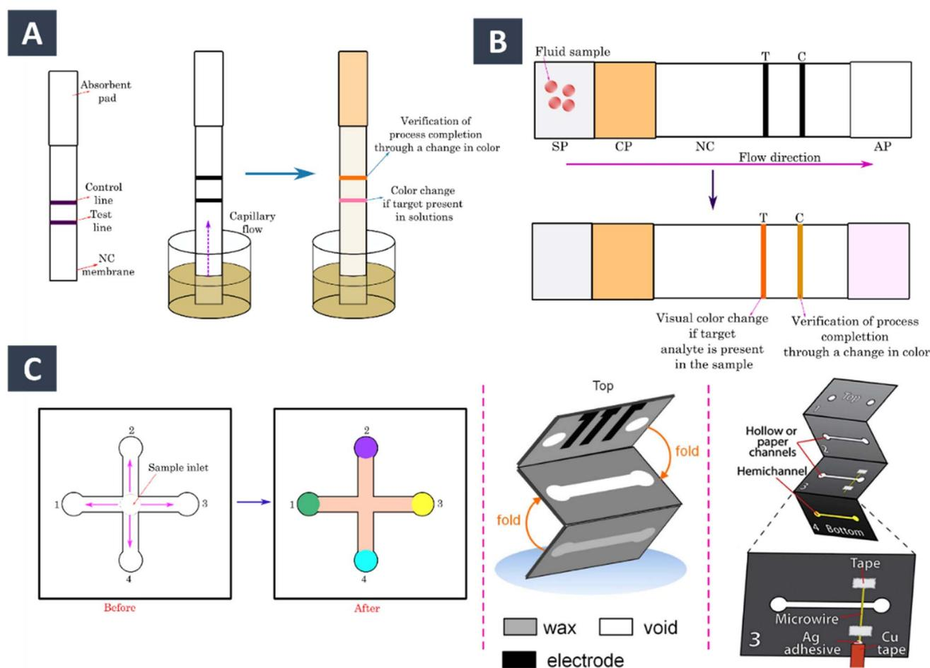
Fig. 8 Schematic illustration of different paper-based assay for biosensing (A) dipsticks comprises of a test line and control line printed on nitrocellulose membrane (B) SP: sample pad, CP: conjugate pad, T: test line, C: control line, and AP: absorbent pad in a lateral flow assays (C) microfluidic device for detecting multiple analytes (left) and an origami-based 3D  $\mu$ PADs.<sup>183,184</sup>
