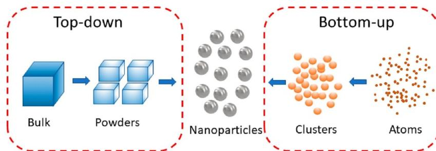
Fig. 4 Bottom-up and top-down methods for synthesizing NMs.<sup>53</sup>
