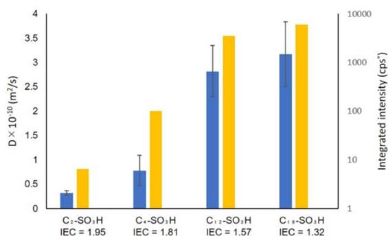
Fig. 6 The self-diffusion coefficient ( $D$ ) of water in  $C_n\text{-SO}_3\text{H}$  (blue) and the integral intensity of the first peak of  $C_n\text{-SO}_3\text{Li}$  in SAXS (yellow). Error bars were calculated from the 95% confidence interval of the linear fitting.
