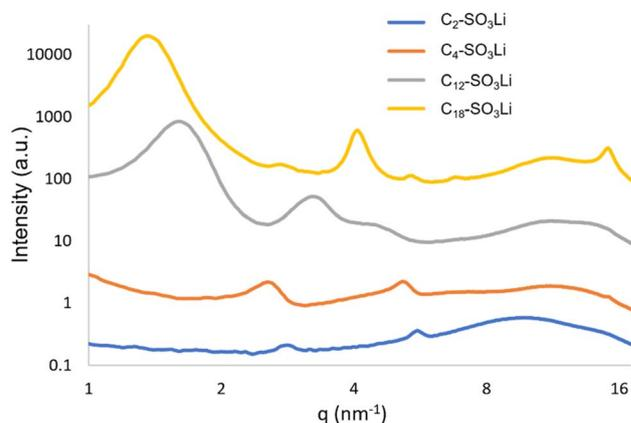
Fig. 3 SAXS profile of  $C_n$ -SO<sub>3</sub>Li.
