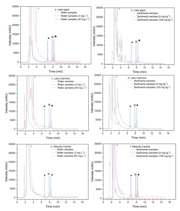
Fig. 8 Chromatograms from the analysis of surface water sample and sediments (\*- benzoyl isocyanate;  $\star$ -7-dehydrocholesteryl-*N*-benzoylcarbamate;  $\boxtimes$ -cholesteryl-*N*-benzoylcarbamate, and  $\blacktriangle$ -coprostanolyl-*N*-benzoylcarbamate).
