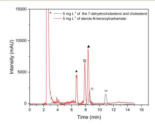
Fig. 6 Chromatograms of sterols in the absence and the presence of the derivatization reaction (\*– benzoyl isocyanate;  $\star$ -7-dehydrocholesteryl-N-benzoylcarbamate;  $\boxtimes$ -cholesteryl-N-benzoylcarbamate, and  $\blacktriangle$ -coprostanolyl-N-benzoylcarbamate  $\odot$  – 7-dehydrocholesterol and  $\infty$  – cholesterol).
