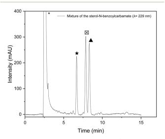
Fig. 2 Chromatogram of the sterols at 3.0 mg L $^{-1}$  after the derivatization reaction, using ACN: ISO (95:5, v/v) at 1.0 mL min $^{-1}$ , 40 °C,  $\lambda$  = 229 nm (\*– benzoyl isocyanate;  $\star$ -7-dehydrocholesteryl-N-benzoylcarbamate;  $\boxtimes$ -cholesteryl-N-benzoylcarbamate, and  $\blacktriangle$ -coprostanolyl-N-benzoylcarbamate).
