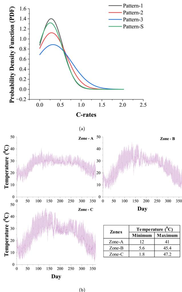
**Fig. 2** (a) Normal probability density function (pdf) distribution of different C-rates across four driving patterns. (b) Temperature profiles of three climatic zones across India for the year 2022 alongside their respective extreme temperature limits.
