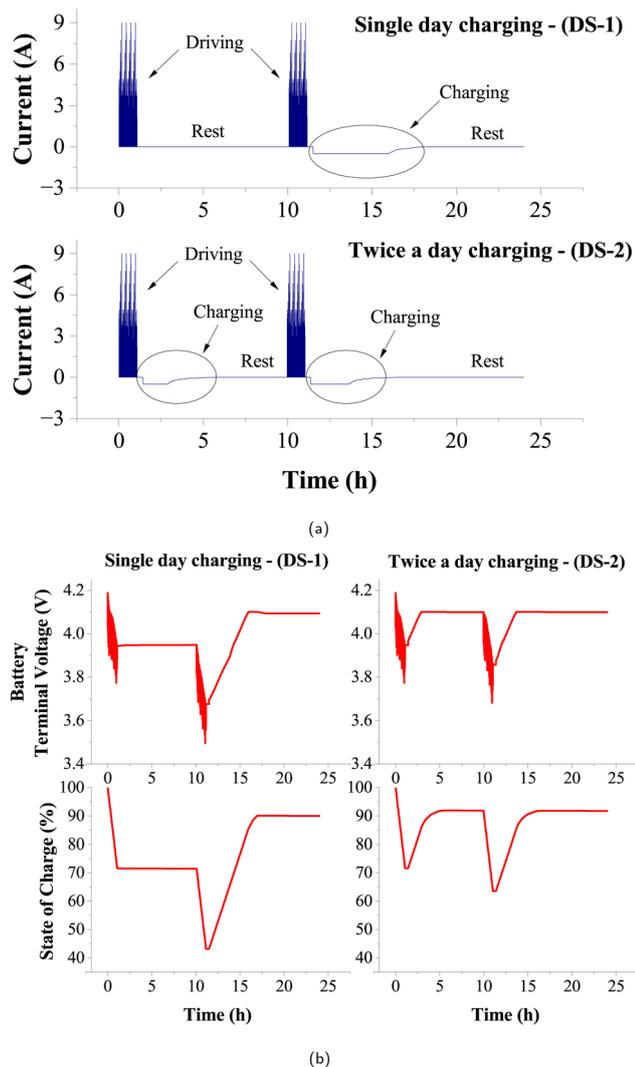
Fig. 3 (a) Two daily scenarios illustrate all the possible phases in an EV's daily cycle. (b) State of charge (SOC) and terminal voltage profiles vary daily for the two daily scenarios.
