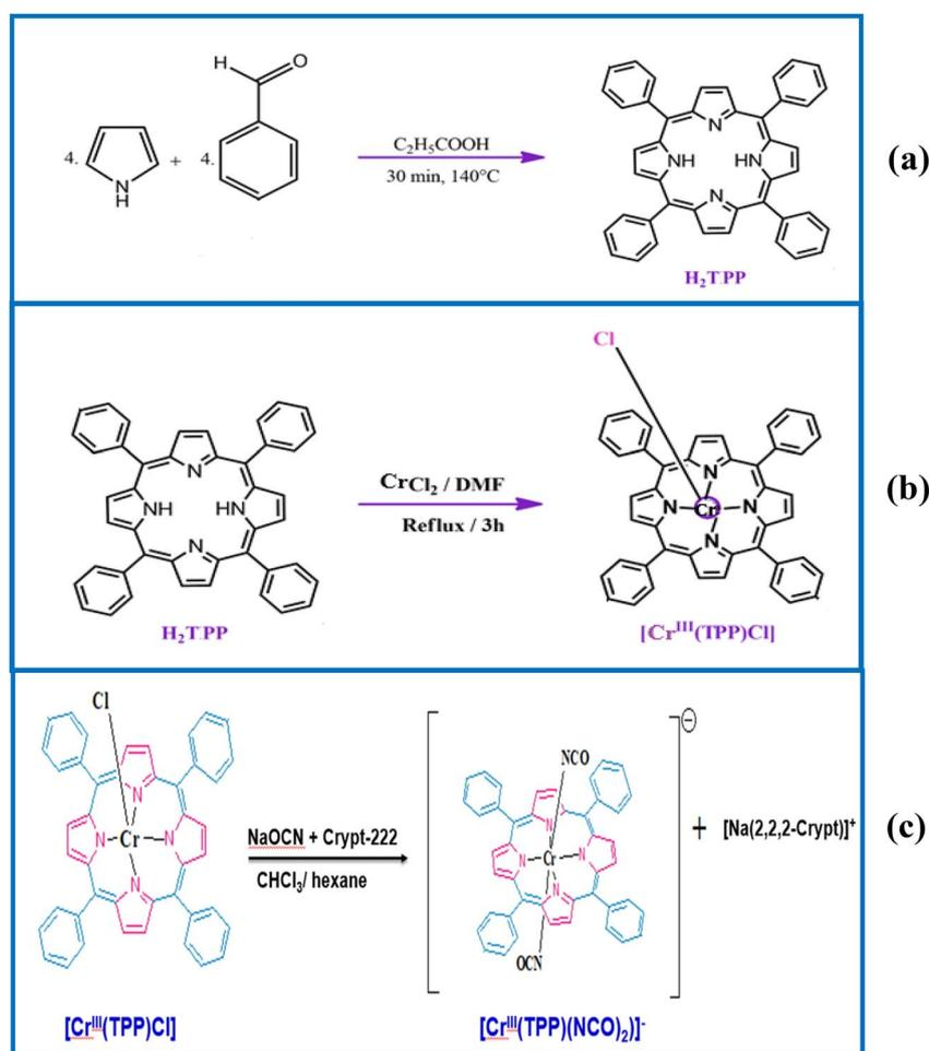
Scheme 1 Synthesis of (a) H<sub>2</sub>TPP, (b) [Cr(TPP)Cl] and (c) [Na(2,2,2-crypt)][Cr(TPP)(NCO)<sub>2</sub>].
