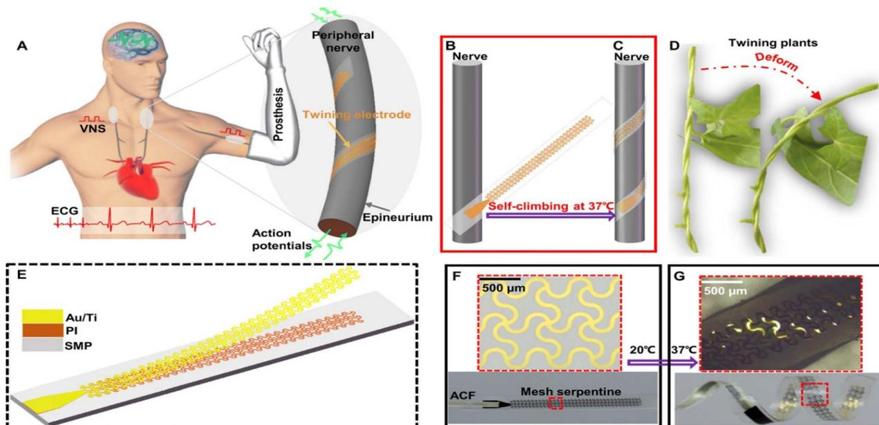
Fig. 5 (A) Pictorial representation of twining electrodes used for peripheral nervous system (PNS); (B and C) self-climbing of SMPs on nerves at 37 °C; (D) representative deformation of the twining plants; (E) design of SMP based twining electrode with Au/Ti and polyimide films; (F) temporary flattened shape of twining electrode; (G) original/ recovered shape of twining electrode (reproduced from ref. 67 with permission from science advances, copyright 2019).
