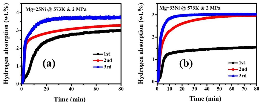
Fig. 5 Hydrogenation behavior of Mg-25Ni (a) and Mg-33Ni (b) alloys synthesized at 573 K and 2 MPa.
