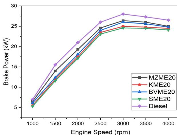
Fig. 3 Brake power variation with engine speed.
