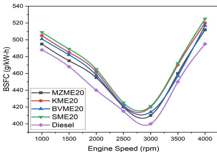
(a) BSFC vs. speed (rpm)
