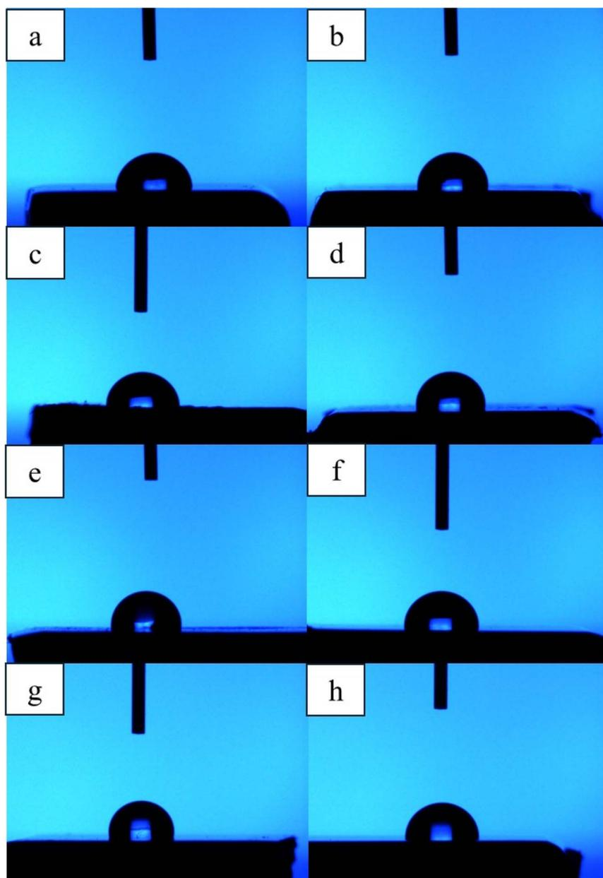
**Fig. 5** Contact angle measurement: (a) UHMWPE, (b–h) UHMWPE/graphene coating with E-beam at 0, 50, 100, 250, and 500 kGy, respectively.
