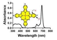
**Fig. 3** Absorption spectrum of Pc. Inset: Chemical structure of a Pc molecule, where "M" denotes the central metal ion and "R" represents the peripheral substituent groups. Reproduced from ref. 30 with permission from Elsevier, copyright © 2021.
