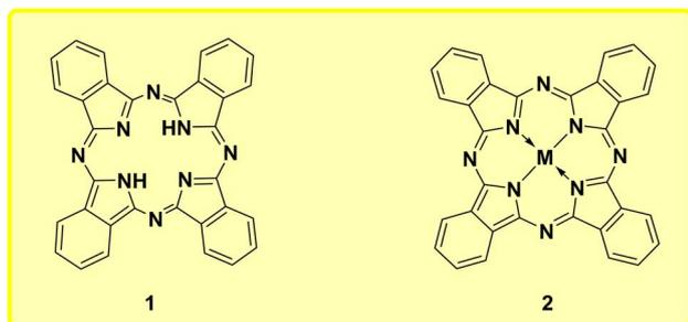
Fig. 2 Structure of phthalocyanine (1) and metal phthalocyanine (2).
