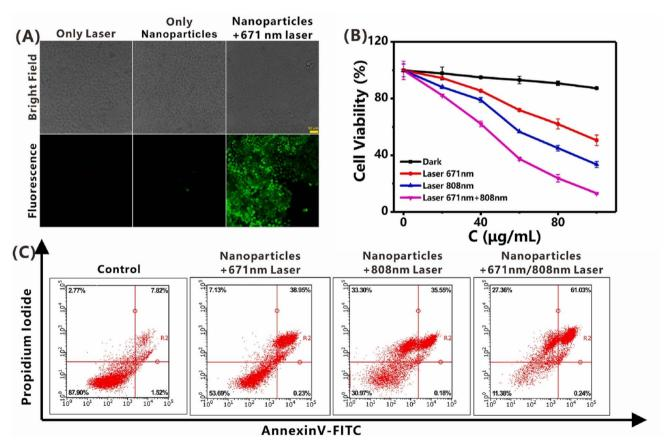
Fig. 28 In vitro evaluation of PDT and PTT effects of TPA-BPAF-SiPc@AuNR@SiO $_2$  in MCF-7 cells. (A) Confocal images showing intracellular ROS generation before and after 671 nm laser irradiation using CM-H2DCFDA probe. (B) Phototoxicity assessed by CCK-8 at varying nanoparticle concentrations. (C) Flow cytometry analysis of apoptosis following treatment with NPs and 671 nm and/or 808 nm laser irradiation. Reproduced from ref. 72 with permission from Elsevier, copyright © 2025.
