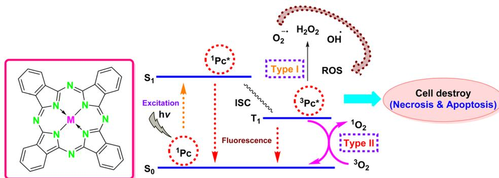
Fig. 1 Schematic representation of the photophysical and photochemical processes involved in PDT, depicted through a modified Jablonski energy level diagram.<sup>14</sup>
