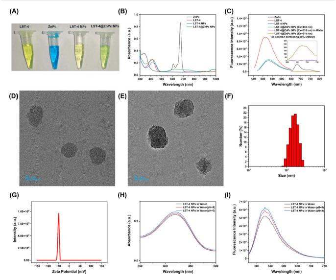
Fig. 22 (A) Images of ZnPc, LST-4, LST-4 NPs, and LST-4@ZnPc NPs. (B) UV-vis spectra and (C) fluorescence intensities of all formulations at 20 μg mL. (D and E) TEM images of LST-4 NPs and LST-4@ZnPc NPs. (F) Size distribution and (G) zeta potential of LST-4@ZnPc NPs. (H and I) pH-dependent UV-vis and fluorescence response of LST-4 NPs. Reproduced from ref. 69, under the terms of the CC BY-NC 3.0 license.
