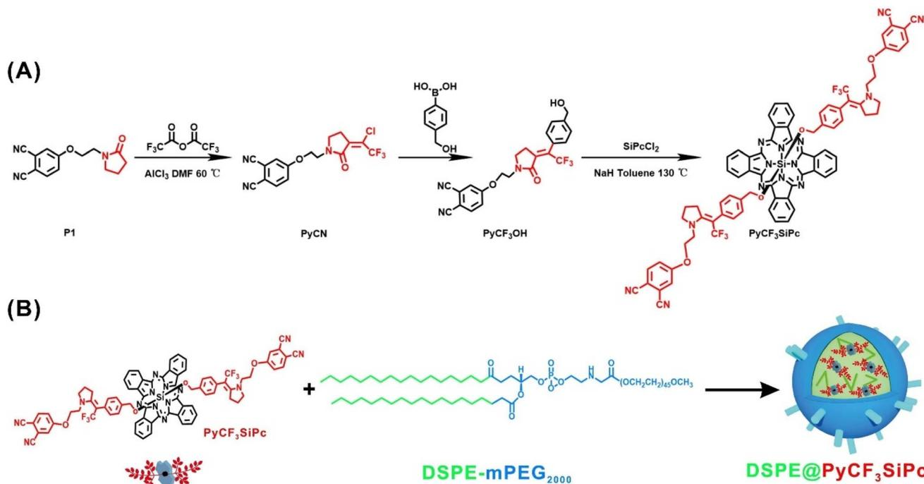
Fig. 34 (A) Synthetic route of  $\text{PyCF}_3\text{SiPc}$  and (B) proposed mechanism for the self-assembly of  $\text{DSPE@PyCF}_3\text{SiPc}$  NPs. Reproduced from ref. 76 with permission from Elsevier, copyright © 2025.
