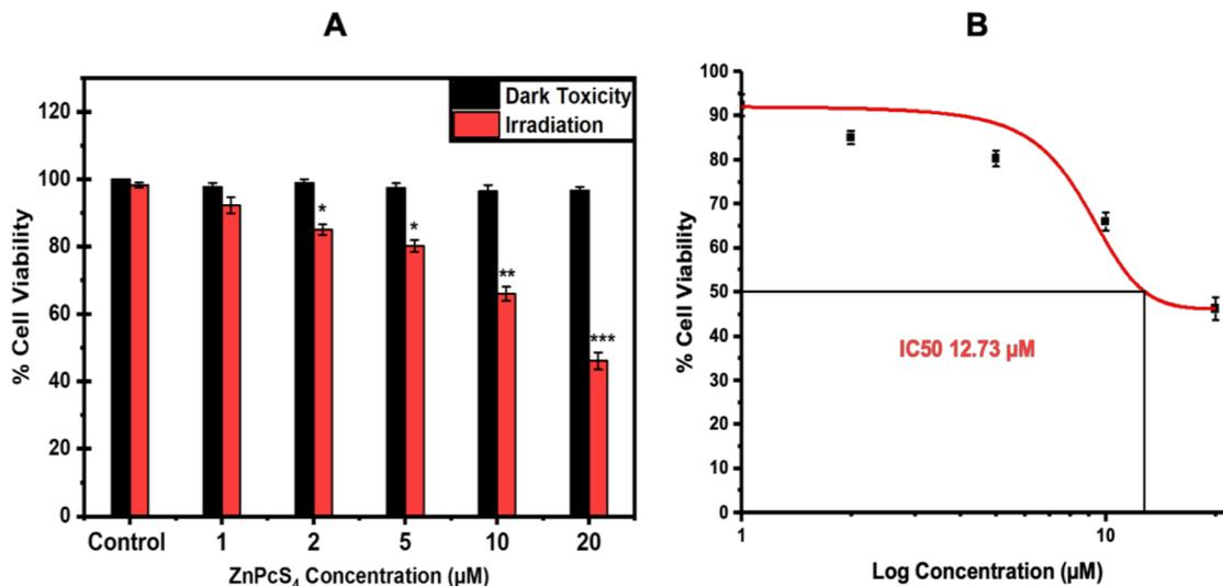
Fig. 11 (A) A375 spheroids treated with increasing concentrations of ZnPcS<sub>4</sub> and photoactivated with a 673 nm laser (10 J cm<sup>-2</sup>). Statistical significance:  $p < 0.05^*$ ,  $p < 0.01^{**}$ ,  $p < 0.001^{***}$  (B) sigmoidal dose–response curve for IC<sub>50</sub> determination. Reproduced from ref. 61, under the terms of the CC BY-NC 3.0 license.
