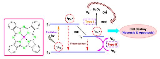
Fig. 1 Schematic representation of the photophysical and photochemical processes involved in PDT, depicted through a modified Jablonski energy level diagram.<sup>14</sup>
