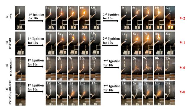
Fig. 5 Photos of UL 94 tests for the fPVC (a), fPVC/MH (b), fPVC/MO@MH (c), and fPVC/MO@MH-PEPE composites (d)
