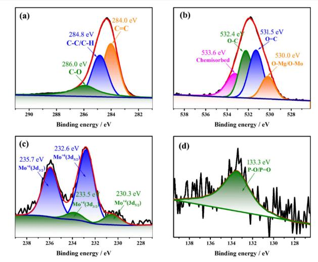
Fig. 9 XPS high-resolution spectra of the inner char residues of fPVC/MO@MH-PEPE composites: (a) C 1s, (b) O 1s, (c) Mo 3d, and (d) P 2p.
