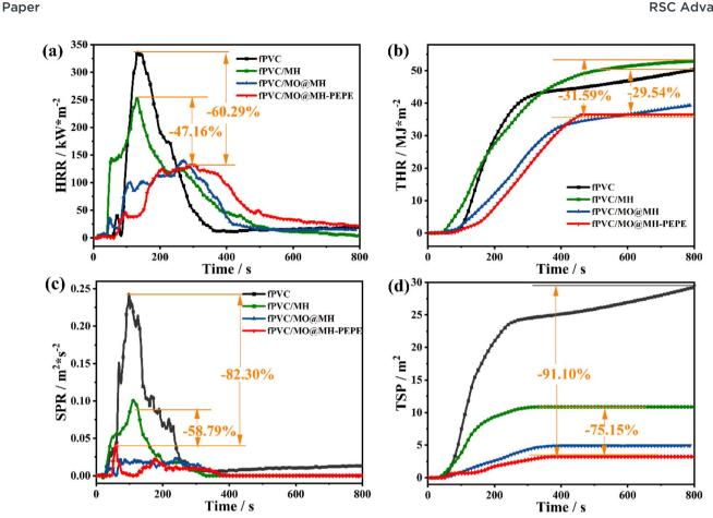
HRR (a), THR (b), SPR (c) and TSP (d) curves of fPVC, fPVC/MH, fPVC/MO@MH, and fPVC/MO@MH-PEPE composites
