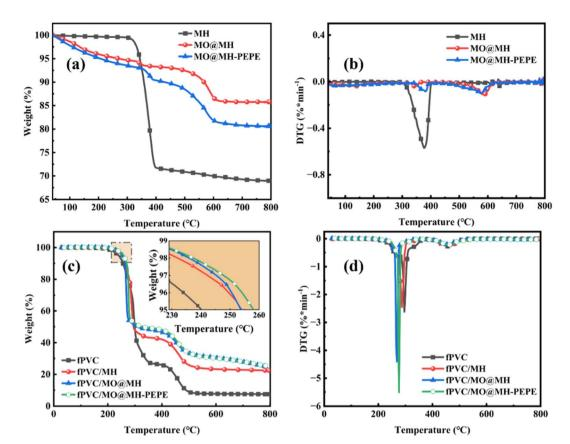
Fig. 4 TG and DTG results of (a) and (b) MH, MO@MH and MO@MH-PEPE (c) and (d) fPVC, fPVC/MH, fPVC/MO@MH and fPVC/MO@MH-PEPE in N<sub>2</sub> atmosphere.
