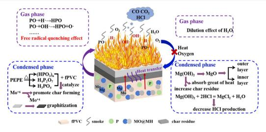
Fig. 11 Schematic illustration of the mechanism for the enhanced flame resistance and smoke suppression of the fPVC/MO@MH-PEPE composite.
