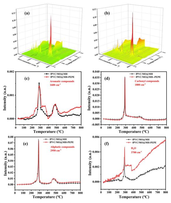
Fig. 10 (a) 3D infrared spectra of fPVC/MO@MH and (b) fPVC/MO@MH-PEPE composites; the intensity changes of (c) aromatic compounds, (d) carbonyl compounds, and (e) aliphatic compounds, (f)  $H_2O$  produced by cracking.
