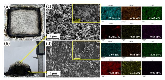
Fig. 7 Photos of char residues of the fPVC/MO@MH-PEPE composites (a) and (b); SEM and EDS images of the outer (c) and inner (d) char residues of the fPVC/MO@MH-PEPE composites.
