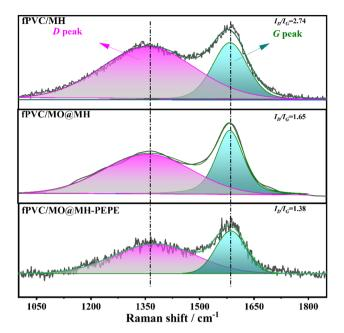
Fig. 8 Raman spectra of the inner char residues of fPVC/MH, fPVC/MO@MH and fPVC/MO@MH-PEPE composites.
