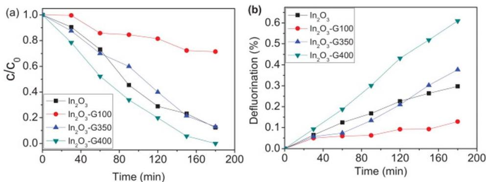
Fig. 20 (a) Photocatalytic decomposition and (b) defluorination of PFOA.<sup>363</sup> "Reproduced from ref. 363 with permission from [Elsevier], copyright [2013]."
