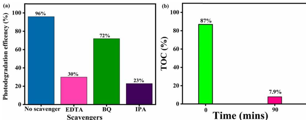
Fig. 28 (a) Reactive species trapping analysis and (b) TOC measurement results for 5% Sm-doped ZnO.<sup>397</sup> "Reproduced from ref. 397 with permission from [Elsevier], copyright [2022]."
