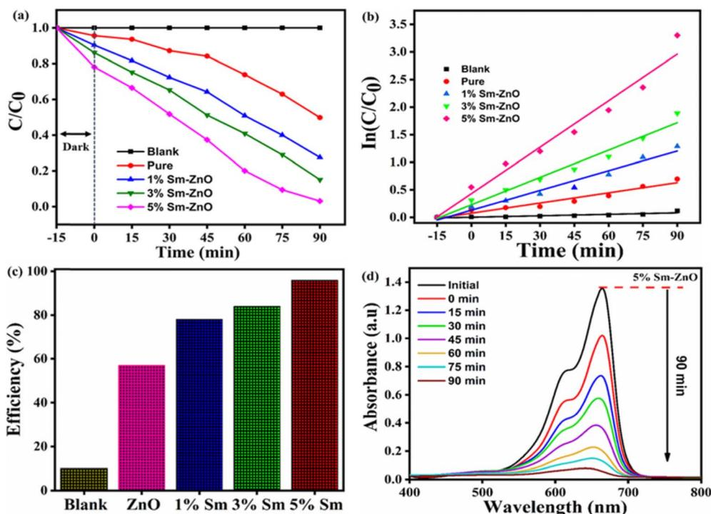
Fig. 27 (a) Variation in MB dye concentration with time, (b) kinetic plot of  $\ln(C/C_0)$ , (c) efficiency of MB degradation by the catalyst, and (d) UV-vis absorption spectra of MB after treatment with 5% Sm-ZnO.<sup>397</sup> "Reproduced from ref. 397 with permission from [Elsevier], copyright [2022]."
