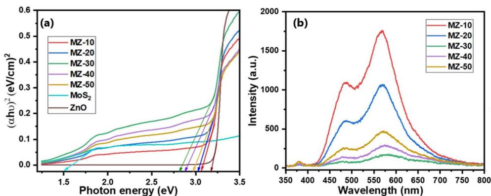
Fig. 34 (a) Bandgap plots of pure ZnO, MoS<sub>2</sub> and ZnO/MoS<sub>2</sub> hybrid, (b) PL spectra of ZnO/MoS<sub>2</sub> hybrid.<sup>426</sup> "Reproduced from ref. 426 with permission from [Elsevier], copyright [2023]."
