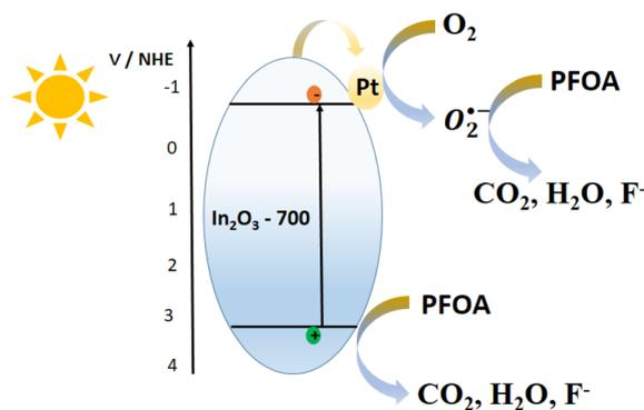
**Fig. 19** Mechanisms highlight the photodegradation of PFOA.<sup>362</sup> "Reproduced from ref. 362 with permission from [Elsevier], copyright [2017]."
