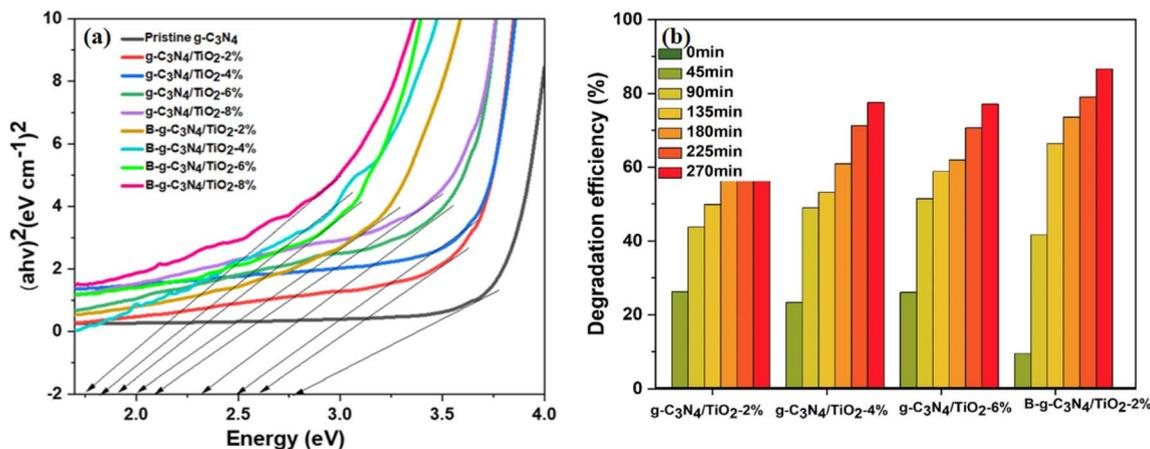
Fig. 26 (a) Bandgap analysis of g-C<sub>3</sub>N<sub>4</sub>, CNT-2%, CNT-4%, CNT-6%, CNT-8%, and BCNT-x composites; (b) evaluation of the photocatalytic degradation efficiency of g-C<sub>3</sub>N<sub>4</sub>/TiO<sub>2</sub>-X (X = 2%, 4%, 6%) compared to B-doped g-C<sub>3</sub>N<sub>4</sub>/TiO<sub>2</sub>-2%.<sup>396</sup> "Reproduced from ref. 396 with permission from [Elsevier], copyright [2023]."
