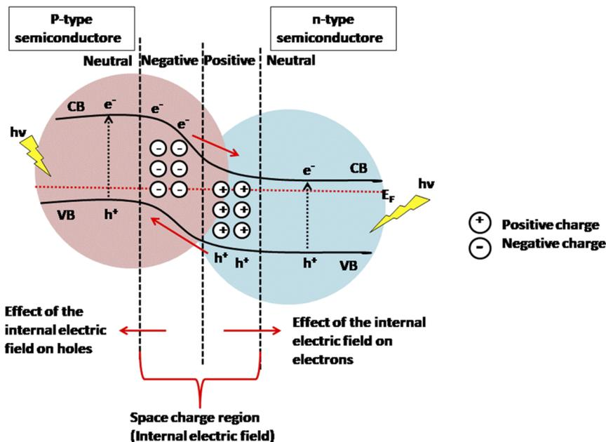
Fig. 17 Diagram showing electron–hole separation under light exposure in a p–n heterojunction photocatalyst.<sup>288</sup>
