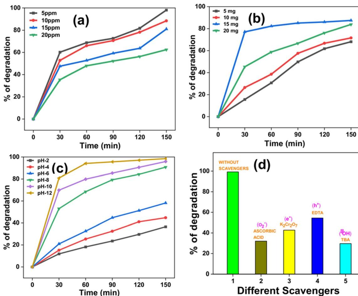
Fig. 30 Influence of (a) dye concentration, (b) catalyst dosage, (c) pH of the solution, and (d) role of various scavengers during MB degradation using CuO-NiO nanocomposite.<sup>399</sup> "Reproduced from ref. 399 with permission from [Elsevier], copyright [2023]."
