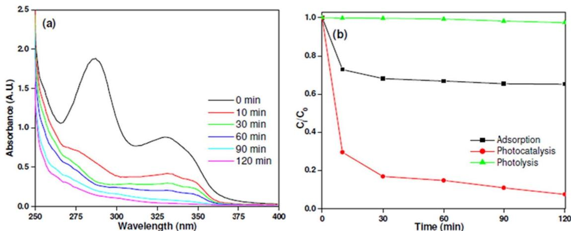
Fig. 31 (a) Absorbance spectra of ofloxacin ( $25 \text{ mg L}^{-1}$ , pH 7) as a function of time using  $0.5 \text{ g L}^{-1}$  catalyst dose; (b) comparative analysis of ofloxacin removal via photocatalysis, photolysis (solar light only), and adsorption (in dark conditions).<sup>424</sup> "Reproduced from ref. 424 with permission from [Elsevier], copyright [2016]."
