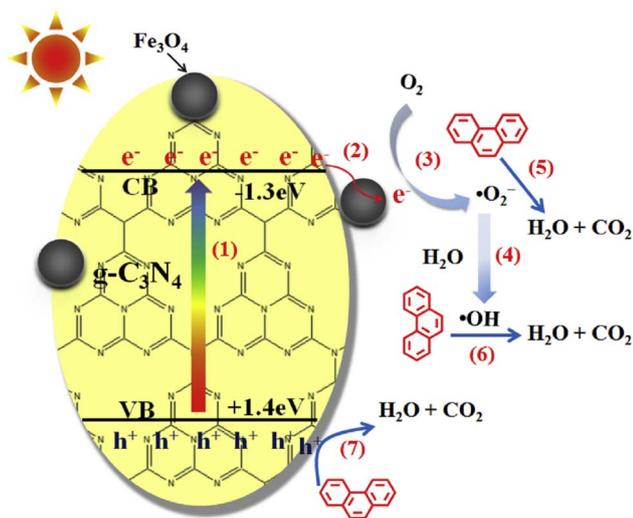
Fig. 23 Proposed schematic mechanism illustrating the transfer and separation of photoinduced charge carriers in the g-C<sub>3</sub>N<sub>4</sub>/Fe<sub>3</sub>O<sub>4</sub> composite under visible light irradiation, highlighting the generation of reactive species responsible for enhanced photocatalytic activity.<sup>366</sup> "Reproduced from ref. 366 with permission from [Elsevier], copyright [2019]."
