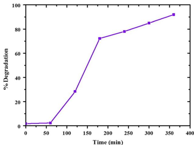
Fig. 25 Percentage degradation of MB dye over time with TiO<sub>2</sub> material.<sup>395</sup> "Reproduced from ref. 395 with permission from [Elsevier], copyright [2021]."
