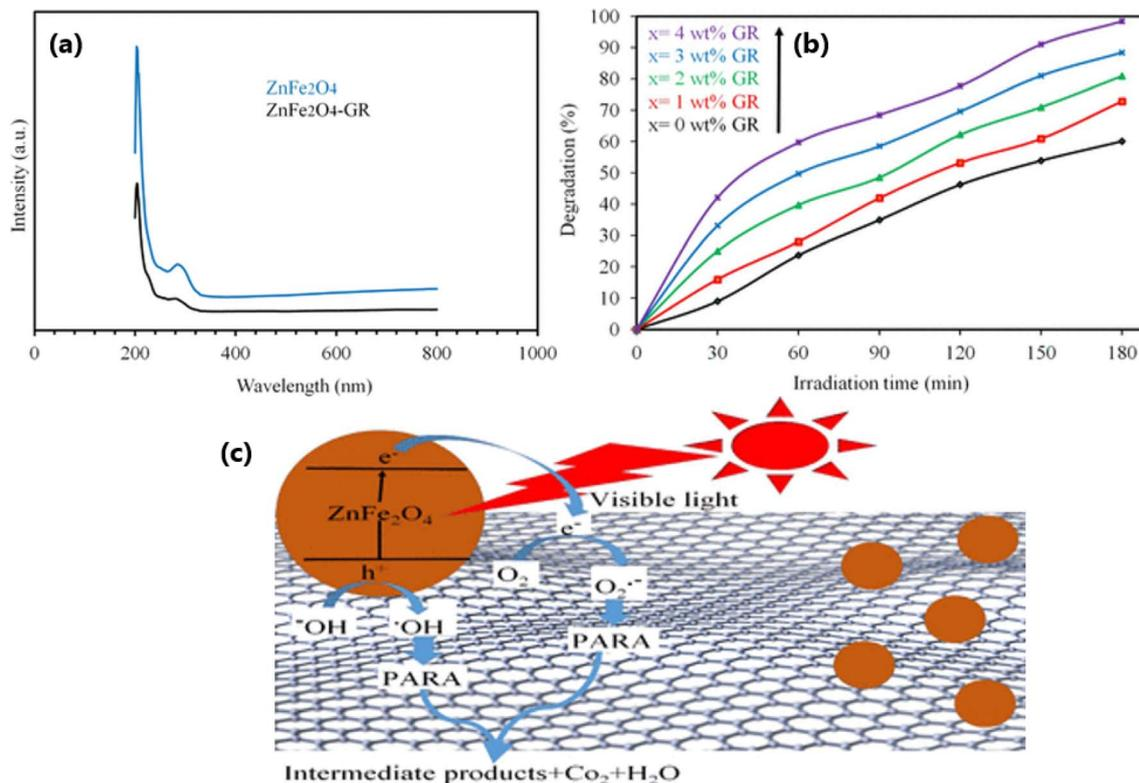
Fig. 33 (a) PL spectra of the pure and hybrid material, (b) photodegradation of paracetamol under visible light, and (c) mechanism of photo-degradation of paracetamol using the composite.<sup>425</sup>
