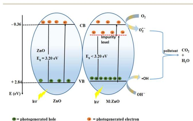
Fig. 15 Diagram showing the introduction of impurities in ZnO photocatalysis.<sup>256</sup> "Reproduced from ref. 256 with permission from [John Wiley and Sons], copyright [2019]."
