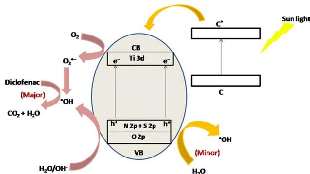
Fig. 14 Diagram showing how C–S–N-tri doped TiO<sub>2</sub> photocatalyst increases photoactivity.<sup>246</sup> Reproduced from ref. 246 with permission from [Elsevier], copyright [2017].
