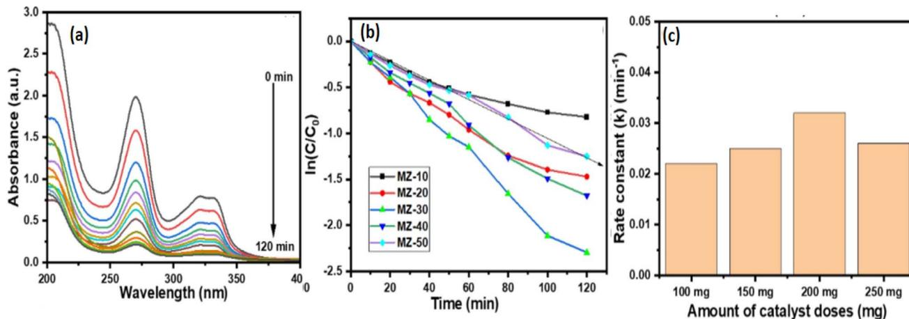
Fig. 35 (a) Excitation spectra of ciprofloxacin antibiotic using 30%-MoS<sub>2</sub>/ZnO sample, (b) plot of  $\ln(C/C_0)$  vs. time, and (c) rate constant values for varying amounts of catalyst dosage.<sup>426</sup> "Reproduced from ref. 426 with permission from [Elsevier], copyright [2023]."
