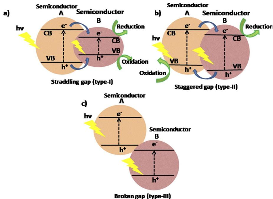
Fig. 16 Diagram showing the separation of electron–hole pair in three types of conventional heterojunction photocatalysts: (a) type-I, (b) type-II, and (c) type-III.<sup>274</sup>
