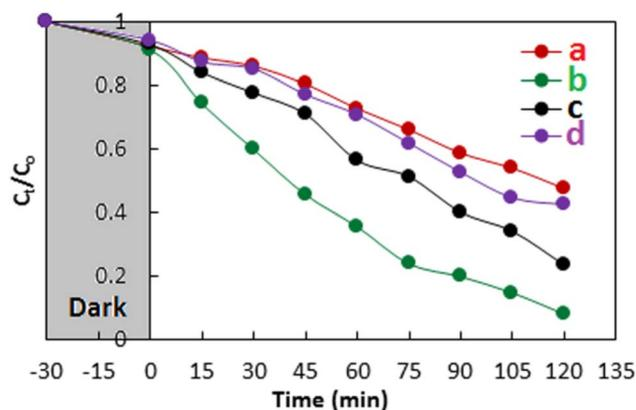
Fig. 29 Photocatalytic degradation of crystal violet dye (50 mL,  $100\text{ mg L}^{-1}$ ) at  $40^\circ C$  with 0.05 g of catalyst: (a)  $Bi_2O_3$ , (b) 5% Ag- $Bi_2O_3$ , (c) 10% Ag- $Bi_2O_3$ , and (d) 15% Ag- $Bi_2O_3$ .<sup>398</sup>
