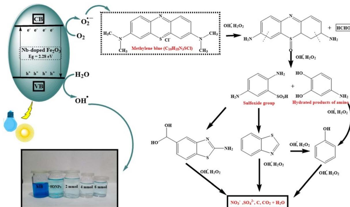
Fig. 12 Mechanism of photodegradation using Nb-doped  $\text{Fe}_2\text{O}_3$ .<sup>198</sup> "Reproduced from ref. 198 with permission from [Elsevier], copyright [2025]."
