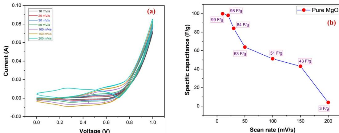
Fig. 8 (a) Different sweep rates of CV for MgONPs electrodes, (b) the variation of the specific capacitance with various scan rates of MgONPs electrode.
