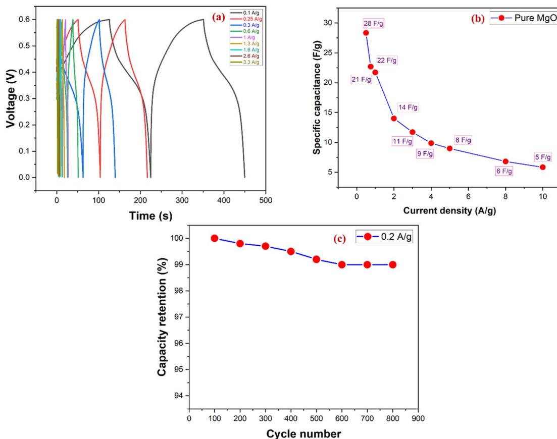
Fig. 9 (a) Different current density of GCD for MgONPs electrodes, (b) the variation of specific capacitance with various current densities of MgONPs electrodes, (c) cyclic performance at  $0.2 \text{ A g}^{-1}$  (800 cycles) with capacity retention.
