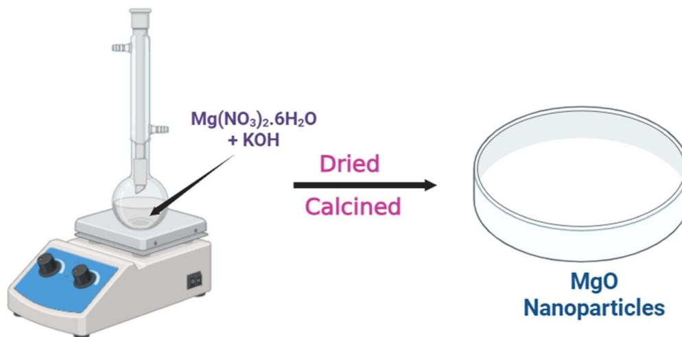
Fig. 1 Synthesis of MgONPs via co-precipitation method.
