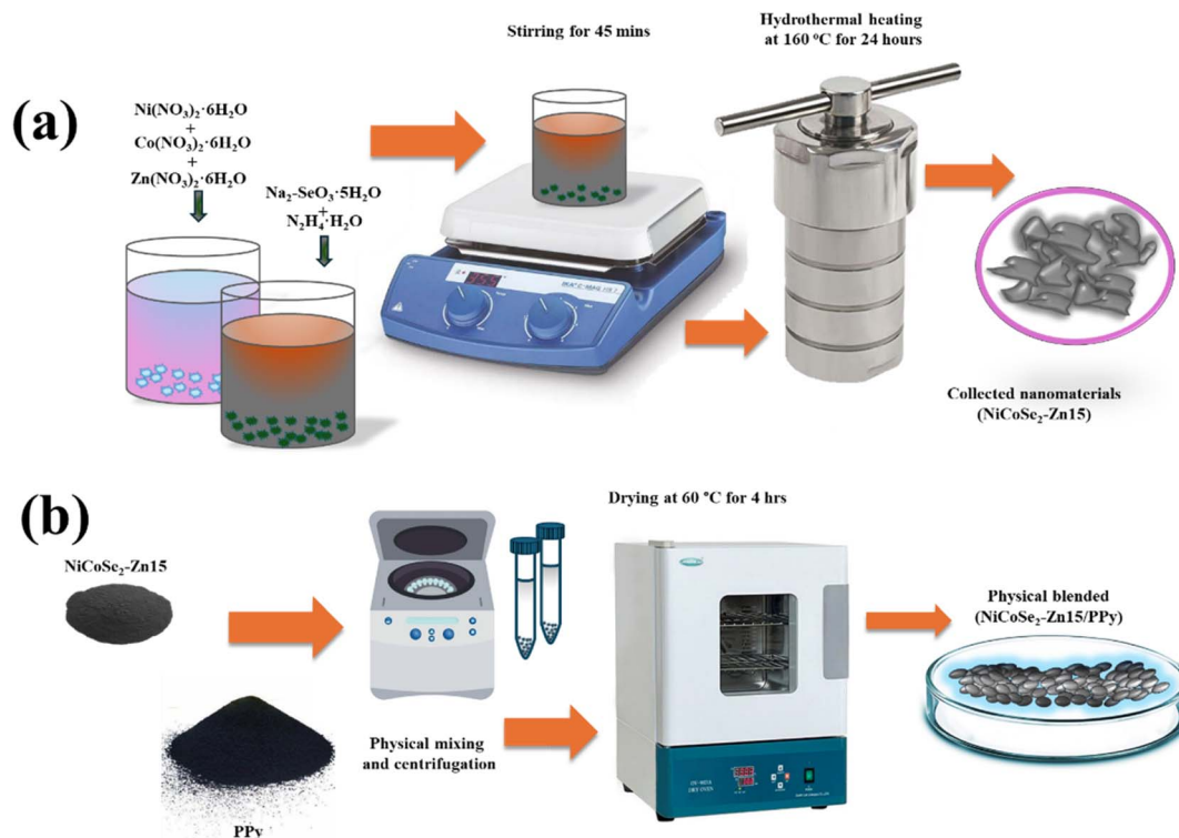
Fig. 1 Schematic overview of the, (a) hydrothermally synthesized NiCoSe 2 -Zn15. (b) Physical mixing of NiCoSe 2 -Zn15 with PPy.
