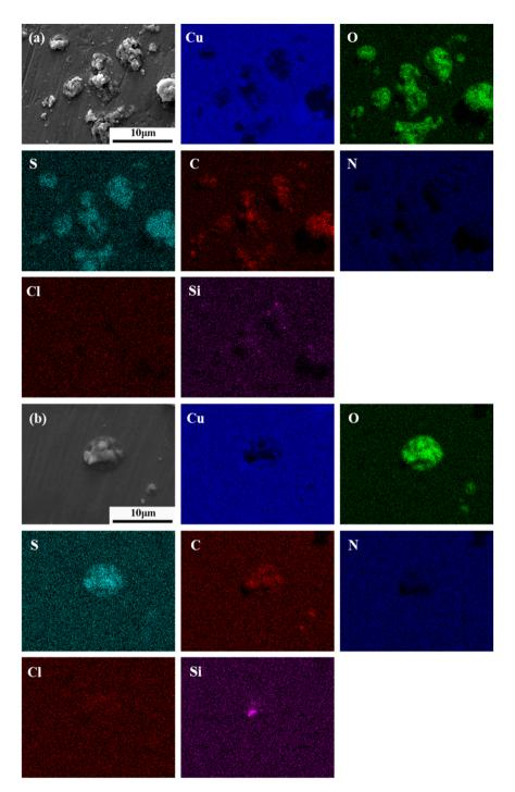
SEM and EDS analysis of PCB-Cu after corrosion induced by (a) 1 μm and (b) 2 μm particles.
