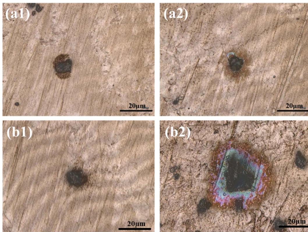
Fig. 4 Surface morphologies of PCB-Cu exposed to (a) 5  $\mu\text{m}$  and (b) 10  $\mu\text{m}$  particles after 1 h (a1 and b1) and 8 h (a2 and b2) of indoor simulated corrosion.
