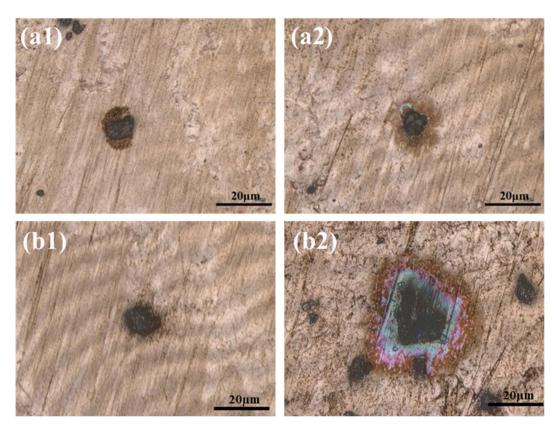
Fig. 4 Surface morphologies of PCB-Cu exposed to (a)  $5 \mu m$  and (b)  $10 \mu m$  particles after 1 h (a1 and b1) and 8 h (a2 and b2) of indoor simulated corrosion.
