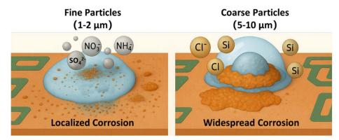
Schematic diagram of particle size and compositions effects on corrosion behavior
