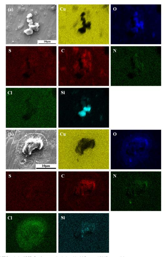
Fig. 6  $\,$  SEM and EDS analysis of PCB-Cu after corrosion induced by (a) 5  $\mu m$  and (b) 10  $\mu m$  particles.
