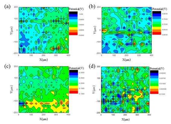
Fig. 8 SKP analysis of corrosion potential distribution on PCB-Cu surfaces after exposure to particles with different sizes: (a) 1  $\mu$ m; (b) 2  $\mu$ m; (c) 5  $\mu$ m; (d) 10  $\mu$ m.
