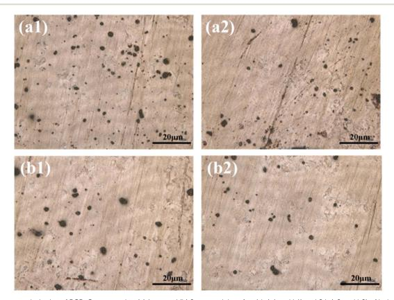
Fig. 3 Surface morphologies of PCB-Cu exposed to (a)  $1 \mu m$  and (b)  $2 \mu m$  particles after 1 h (a1 and b1) and 8 h (a2 and b2) of indoor simulated corrosion.
