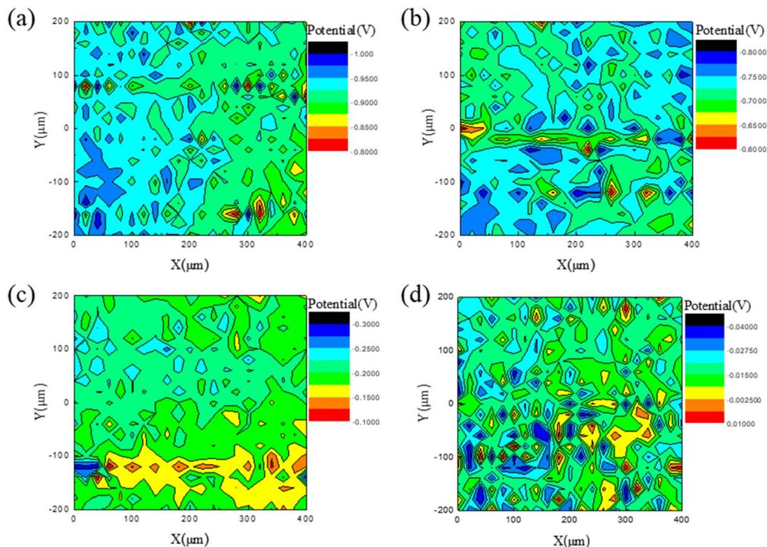
Fig. 8 SKP analysis of corrosion potential distribution on PCB-Cu surfaces after exposure to particles with different sizes: (a) 1  $\mu\text{m}$ ; (b) 2  $\mu\text{m}$ ; (c) 5  $\mu\text{m}$ ; (d) 10  $\mu\text{m}$ .
