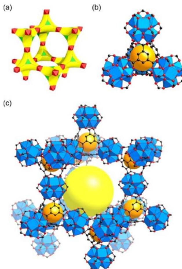
**Fig. 15** Schematic of the **spn** topology (a) exhibited by **MOF-808** with two kind of cages, first octahedral which indicate with red, and triangular which showed with green. (b) and large adamantane pores (c) atom color scheme: black for carbon, red for oxygen, blue for Zr. H atoms are hidden for better understanding. Large yellow and small orange balls showed the space in the framework.<sup>133</sup> From ref. 132 with permission. Copyright 2015, Wiley-VCH.
