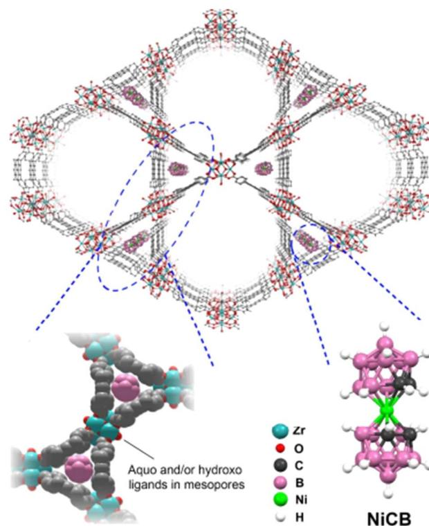
Fig. 5 The crystalline structure of **NiCB@NU-1000** with occupied triangular channels and lack of hydrogen atoms. Triangular shaped channels of **NiCB@NU-1000** are also demonstrated in below to illustrate the close interaction between **NiCB** and three neighbor pyrenes. Also there is presentation of **NiCB**.<sup>109</sup> From ref. 109 with permission. Copyright 2018, American Chemical Society.
