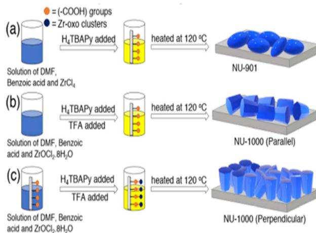
Fig. 12 Synthesis process to solvothermally produce films of three product (a) **NU-901**, (b) **NU-1000** with parallel and (c) perpendicular orientation.<sup>122</sup> From ref. 122 with permission. Copyright 2021, American Chemical Society.
