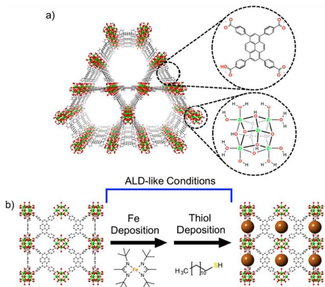
Fig. 3 (a) Structure of the NU-1000 and its 6 metal cluster and pyrene-based linker that includes the binding sites for iron thiolate precipitation and deposition, which are zoomed in (b) the ALD procedure of iron thiol cluster generation in the MOF.<sup>9</sup> From ref. 9 with permission. Copyright 2019, American Chemical Society.
