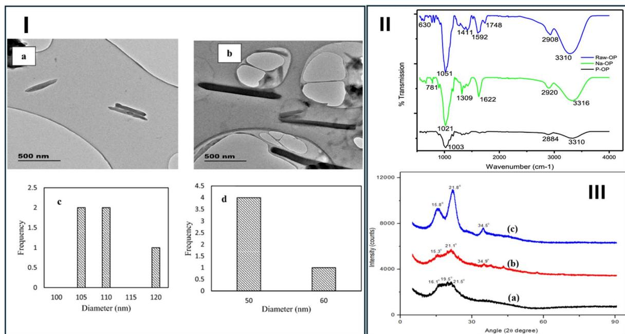
Fig. 36 (I) TEM analysis of unground (a) and milled (b) orange peel, in addition to the particle size distribution histograms of unground (c) and milled (d) orange peel. FTIR (II) and XRD (III) spectra of (a) raw orange peels (OP), (b) alkali-treated orange peels using sodium hydroxide (NaOP), and (c) acid-treated orange peels using phosphoric acid (POP). Reproduced from ref. 124, copyright 2024 Springer Nature.
