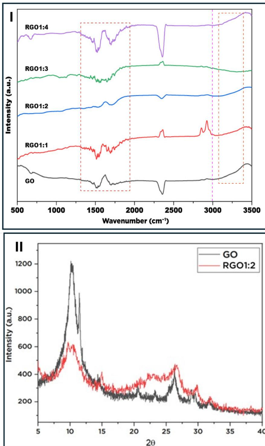
Fig. 24 FTIR (I) and XRD (II) spectra of GO and green synthesized rGO, revealing their chemical and crystalline structures. Reproduced from ref. 114, copyright 2022 MDPI.
