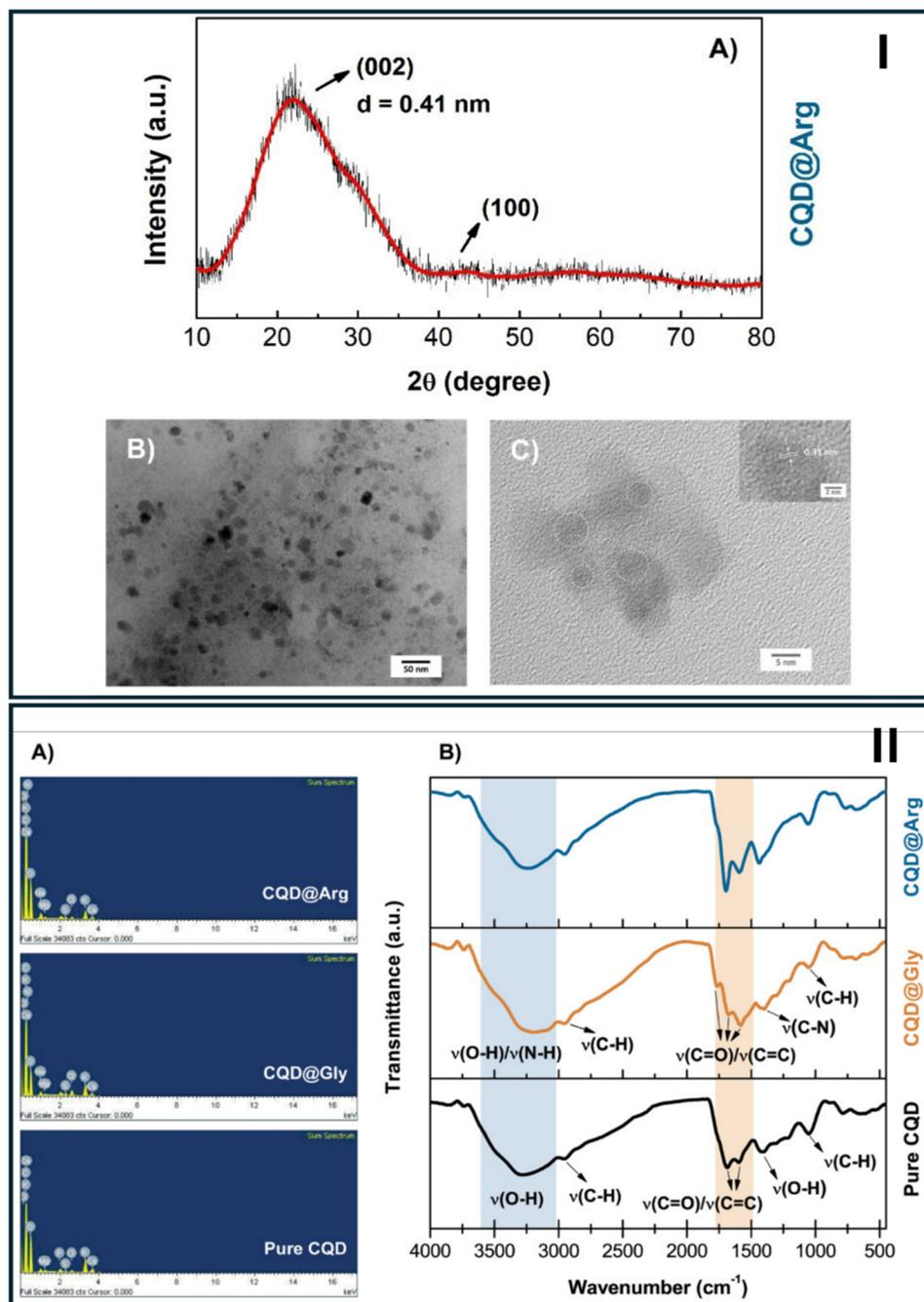
Fig. 26 (I) (A) XRD and (B & C) TEM analyses of CQD@Arg NPs exhibiting lattice spacing of  $d = 0.31$  nm. (II) (A) EDS and (B) FTIR spectra of CQDs and N-CQDs. Reproduced from ref. 115, copyright 2021 MDPI.
