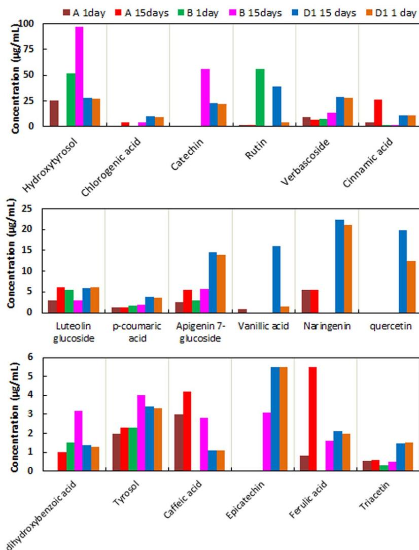
Fig. 8 Identification and quantification of migrated phenolic compounds and triacetin from PLA 8% film into different food simulants based on HPLC-DAD analysis.
