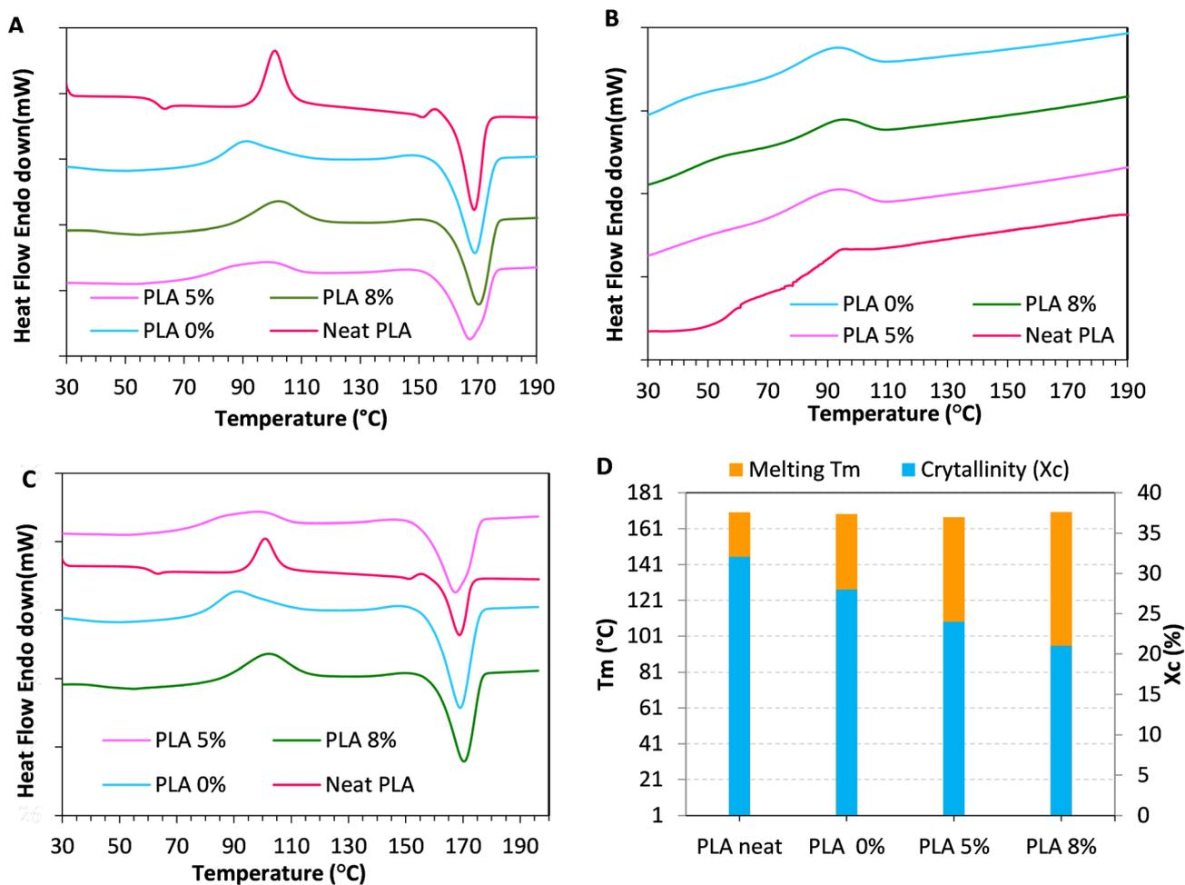
Fig. 2 DSC analysis data: (A) first heating scans, (B) cooling plots, (C) second heating scans, and (D) melting temperature and degree of crystallinity  $X_c$  after the first and second scans of neat PLA, PLA 0%, PLA 5% and PLA 8%.
