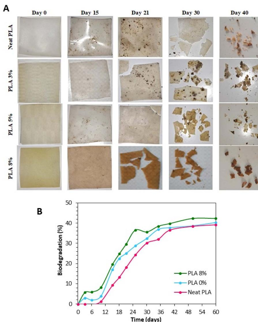
Fig. 9 (A) Visual images of the films after different times of burial in soil. (B) Biodegradation test of neat PLA, PLA 0%, PLA 8% films based on the mineralization of carbon at 58 °C.
