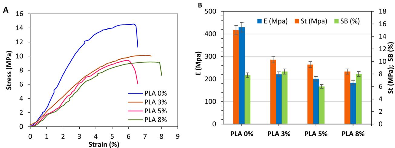
Fig. 1 (A) Stress-strain plots, and (B) strength (*S*), Young's modulus (*E*), and strain at break (*SB*) of neat PLA and plasticized PLA/OLE films with different OLE contents.
