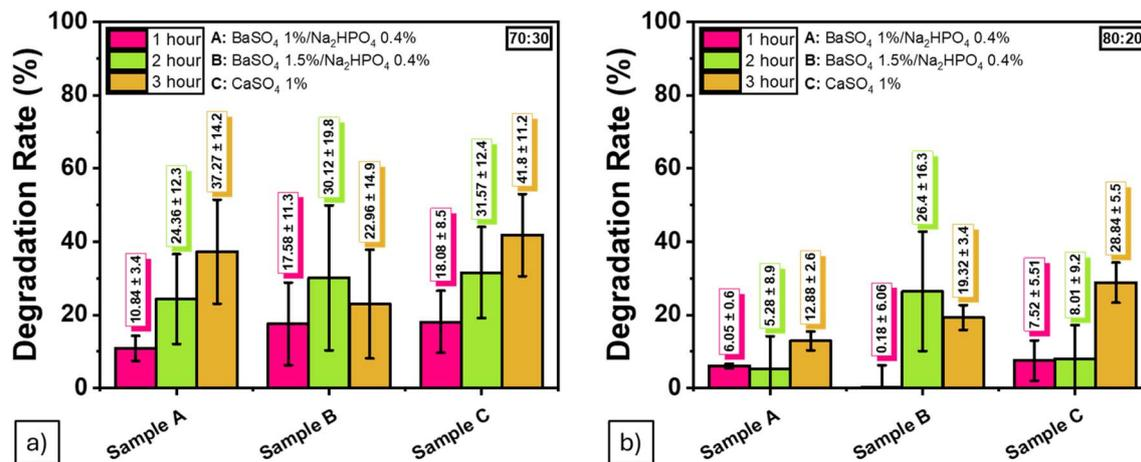
Fig. 13 Initial degradation behavior of ALG/PVA/BaSO<sub>4</sub> hydrogel composites over 5 hours from (a) 70:30, (b) 80:20 ratio (short-term assessment).
