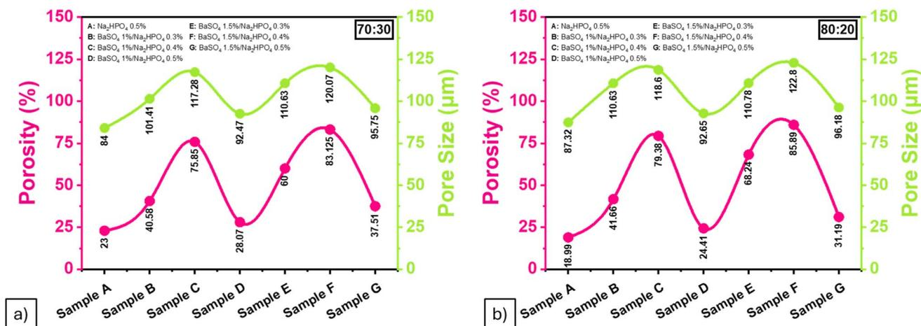
Fig. 6 Percent porosity and pore size of ALG/PVA/BaSO<sub>4</sub> hydrogel composites from (a) 70 : 30, (b) 80 : 20 ratio.
