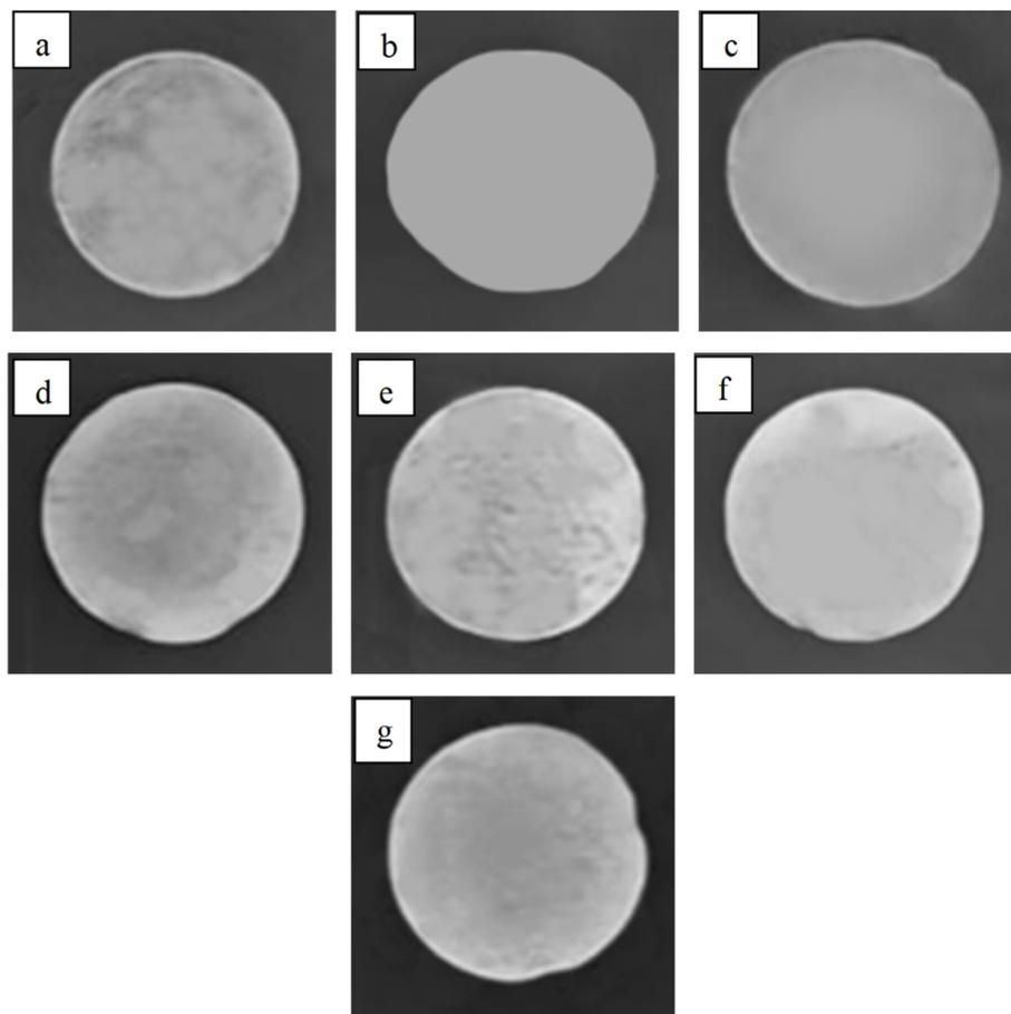
Fig. 8 Results of radiopacity testing on ALG/PVA/BaSO<sub>4</sub> hydrogel variation 70 : 30; (a) Na<sub>2</sub>HPO<sub>4</sub> 0.5%, (b) BaSO<sub>4</sub> 1%/Na<sub>2</sub>HPO<sub>4</sub> 0.3%, (c) BaSO<sub>4</sub> 1%/Na<sub>2</sub>HPO<sub>4</sub> 0.4%, (d) BaSO<sub>4</sub> 1%/Na<sub>2</sub>HPO<sub>4</sub> 0.5%, (e) BaSO<sub>4</sub> 1.5%/Na<sub>2</sub>HPO<sub>4</sub> 0.3%, (f) BaSO<sub>4</sub> 1.5%/Na<sub>2</sub>HPO<sub>4</sub> 0.4%, (g) BaSO<sub>4</sub> 1.5%/Na<sub>2</sub>HPO<sub>4</sub> 0.5%.
