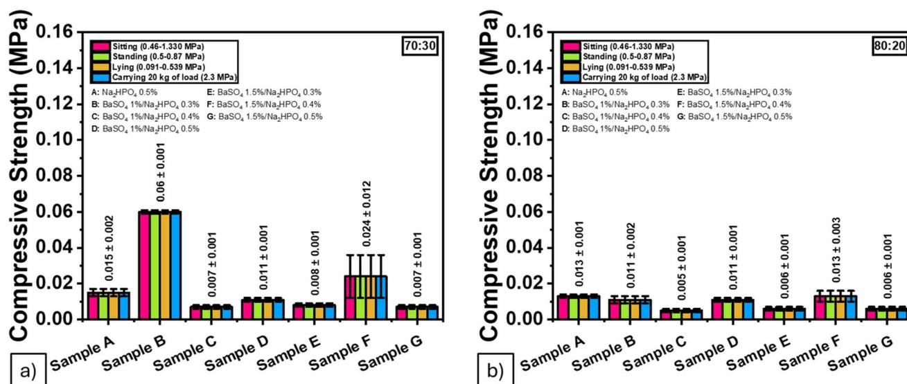
**Fig. 10** Compressive strength values of the ALG/PVA/BaSO<sub>4</sub> hydrogel composite from (a) 70 : 30, (b) 80 : 20 ratio.
