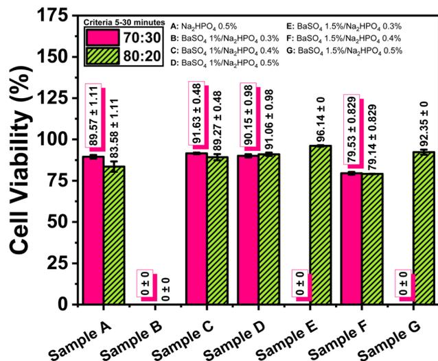
Fig. 11 Effect of BaSO<sub>4</sub> and Na<sub>2</sub>HPO<sub>4</sub> on cell viability of the ALG/PVA hydrogel composite.
