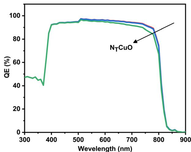
Fig. 11 Quantum efficiency versus wavelength of CuO solar cell with various  $N_T$  (CuO).
