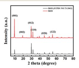
Fig. 3 XRD pattens of BiOl.
