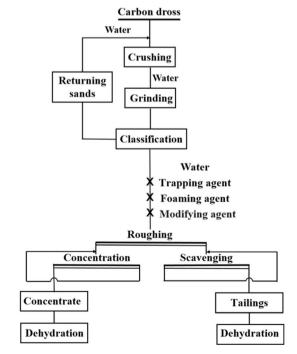
Fig. 7 Flotation process for carbon dross.
