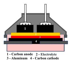
Fig. 3 Structure of an aluminum electrolysis cell. 14
