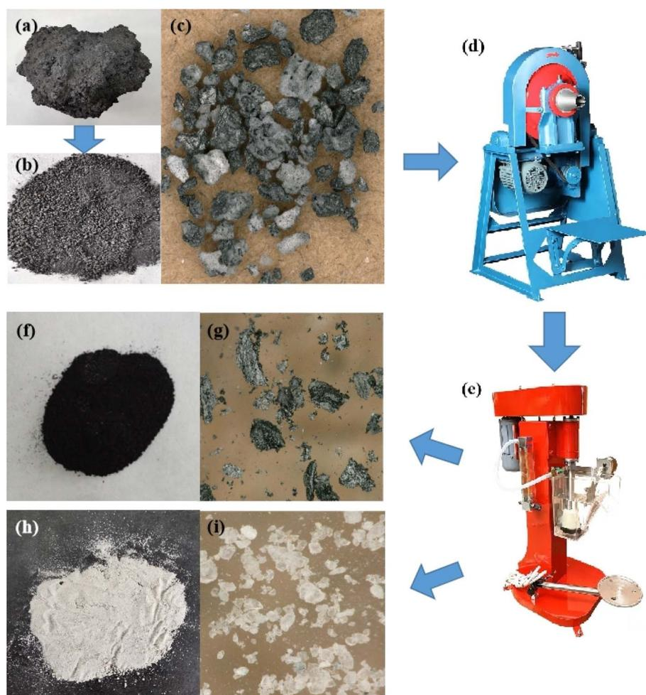
Fig. 5 Diagram of the carbon dross flotation experimental process and product. (a) Massive carbon dross salvaged from the aluminium electrolytic cell. (b) Crushed carbon dross. (c) Crushed carbon dross under an ultra-depth three-dimensional microscope (UTMS). (d) Conical ball mill. (e) Single-cell flotation machine. (f) Carbon powder after flotation. (g) Carbon powder after flotation under UTMS. (h) Electrolytes after flotation. (i) Electrolytes after flotation under UTMS.
