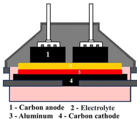
Fig. 3 Structure of an aluminum electrolysis cell.<sup>14</sup>
