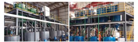
Fig. 8 Carbon dross flotation production line. (a) A 6 kt a<sup>-1</sup> treatment line in Henan, China and (b) a 20 kt a<sup>-1</sup> treatment line in Liaoning, China.
