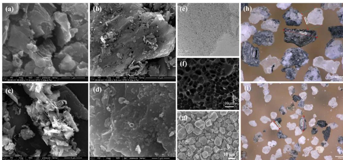
Fig. 9 Morphology and applications of carbon dross. (a)–(d) SEM images of carbon dross from different aluminum electrolytic plants. (e) TEM photograph of carbon catalytic supports;<sup>82</sup> (f) SEM photograph of an efficient carbon-based adsorption material.<sup>85</sup> (g) SEM image of the deoxygenated porous carbon for capacitors.<sup>86</sup> (h) and (i) Ultra-depth three-dimensional microscopy image of mechanically liberated carbon dross.
