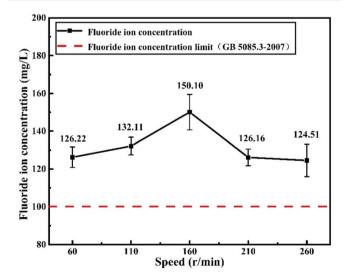
Fig. 6 Fluoride-ion concentrations in the leaching solutions of carbon powder collected from a carbon dross flotation industrial line (note: the shaking speeds specified in "HJ 557-2010" is  $110 \pm 10$  rpm).
