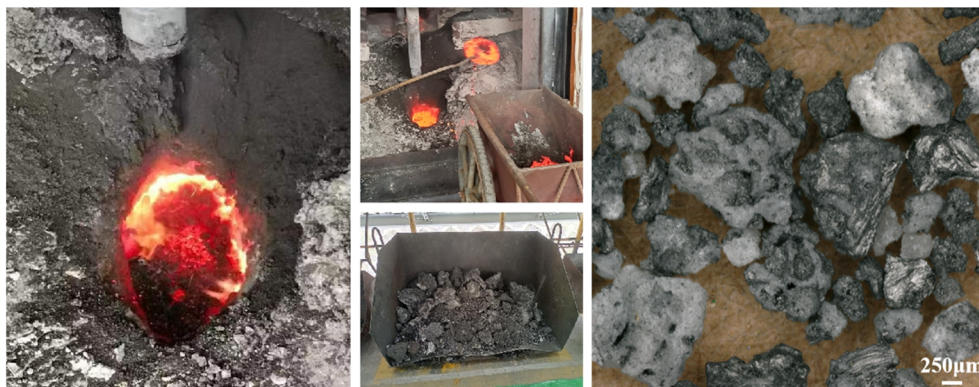
Fig. 1 Removal, temporary storage, and microstructural characterization of carbon dross in an aluminum electrolysis plant in China.
