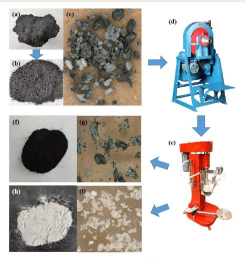
Fig. 5 Diagram of the carbon dross flotation experimental process and product. (a) Massive carbon dross salvaged from the aluminium electrolytic cell. (b) Crushed carbon dross. (c) Crushed carbon dross under an ultra-depth three-dimensional microscope (UTMS). (d) Conical ball mill. (e) Single-cell flotation machine. (f) Carbon powder after flotation. (g) Carbon powder after flotation under UTMS. (h) Electrolytes after flotation under UTMS.
