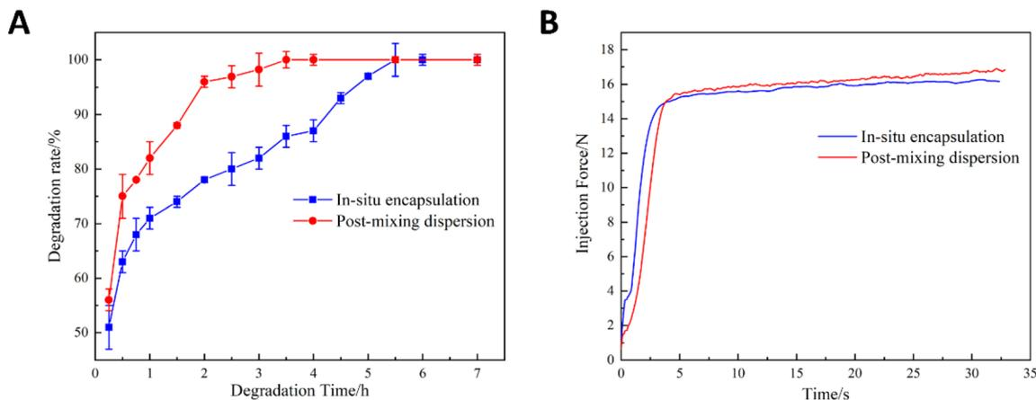
Fig. 8 The degradation behaviors (A) and injection force characterization (B) of the CHPs hydrogels fabricated by *in situ* encapsulation and post-mixing dispersion methods. Error bars denote triplicate measurements ( $n = 3$ ).
