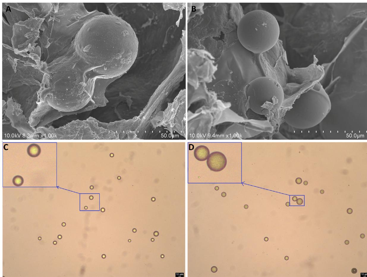
Fig. 6 The morphologies of the PLLA microspheres fabricated by (A and C) *in situ* encapsulation and (B and D) post-mixing dispersion. Images acquired using: (A and B) scanning electron microscopy (SEM); (C and D) optical microscopy.
