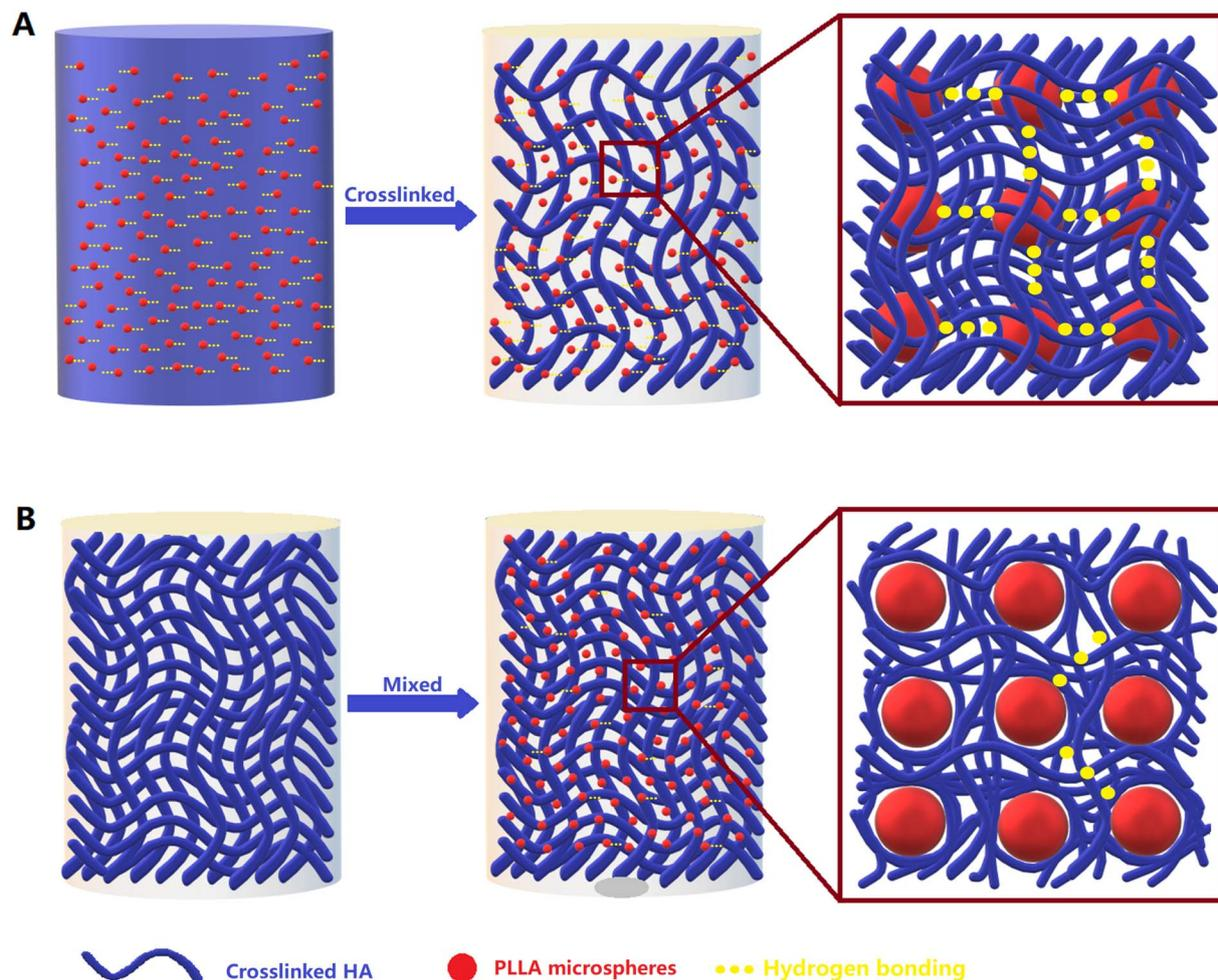
Fig. 5 Schematic illustration of two fabrication strategies for crosslinked HA hydrogels/PLLA microspheres composites (CHP). (A) *In situ* encapsulation: PLLA microspheres embedded within covalently crosslinked HA networks via sequential dispersion and crosslinking; (B) post-mixing dispersion: mechanical blending of PLLA microspheres into pre-crosslinked HA hydrogel matrices.
