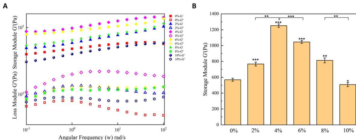
Fig. 2 Rheological behavior and viscoelastic quantification of CHPs modulated by PLLA feed concentration (0–10% w/v). (A) The frequency-dependent viscoelastic profiles. (B) Storage modules ( $G'$ ) magnitudes across concentration gradients. Error bars denote triplicate measurements ( $n = 3$ ). Statistical annotations ( $*p < 0.05$ ,  $**p < 0.01$ ,  $***p < 0.001$ ).
