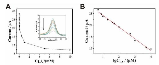
Fig. 5 (A) Response of the aptasensor to different concentrations of lactate (5  $\times$  10<sup>-3</sup> to 10 mM). (B) The linear relationship between DPV intensity and lactate concentration in an exponential range.
