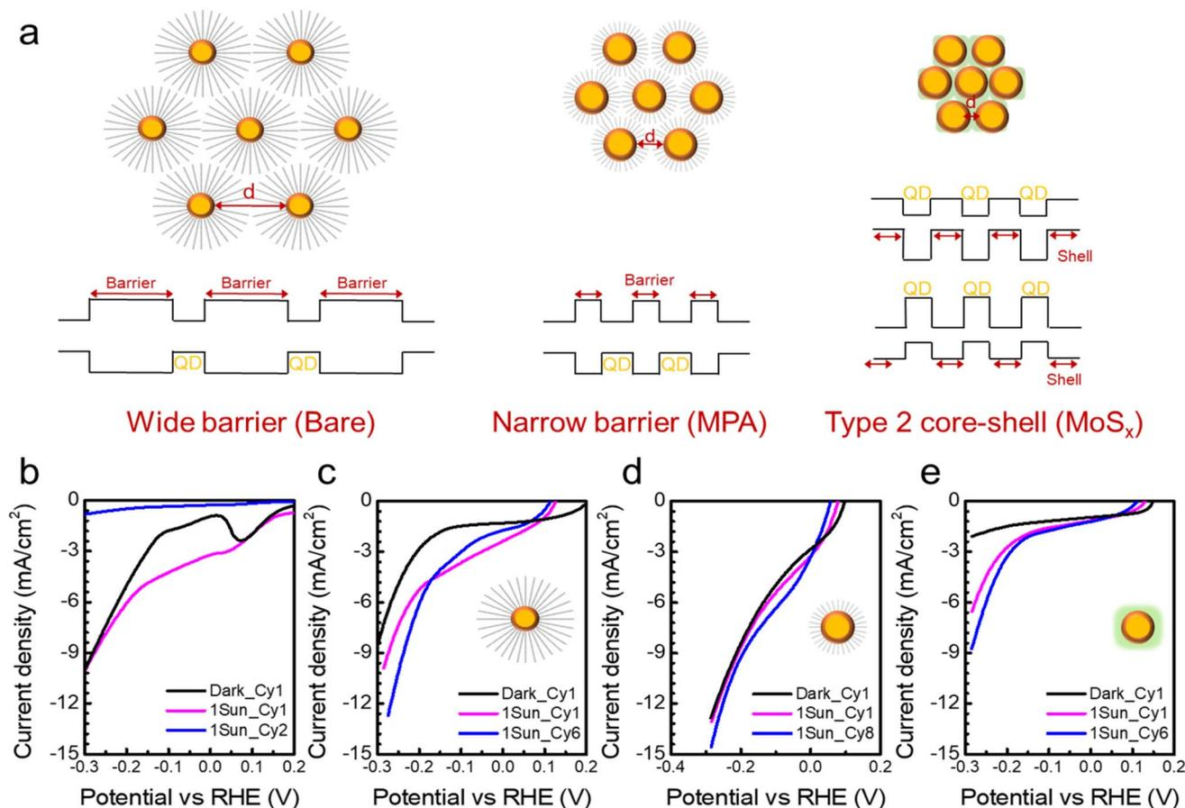
Fig. 1 (a) Schematic illustration of the band alignment of CISE<sub>2</sub> CNCs with different shell systems. (b–e) Current density versus cathodic potential ( $J$ – $V$ ) curves for (b) bare Cu<sub>2</sub>O/CuO, (c) Cu<sub>2</sub>O/CuO/CISE<sub>2</sub> CNCs capped with insulating ligands, (d) Cu<sub>2</sub>O/CuO/CISE<sub>2</sub> CNCs capped with organic linker ligands, and (e) Cu<sub>2</sub>O/CuO/CISE<sub>2</sub> CNCs capped with matrix-type ligands (post-annealing at 250 °C).
