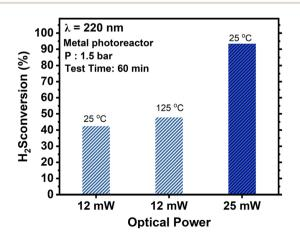
Fig. 4 Effect of laser power and reaction temperature on the photolysis of  $5\%~H_2S$  at 220~nm.
