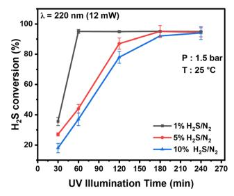
Fig. 3 Photolysis of  $H_2S$  at 220 nm in the metallic photoreactor for different  $H_2S/N_2$  mixtures as a function of reaction (UV illumination) time
