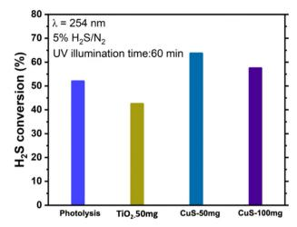
Fig. 8 Comparison of photolytic and photocatalytic batch experiments conducted in the quartz reactor with an Hq lamp.
