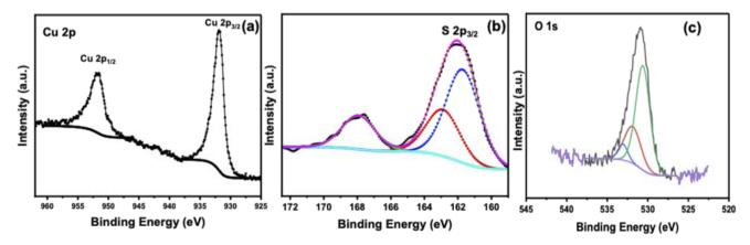
Fig. 10 High-resolution XPS spectra of CuS: (a) Cu 2p region showing Cu valence states, (b) S 2p region confirming  $S^{2-}$  and surface  $S^{0}$  species, and (c) O 1s region indicating adsorbed hydroxyl groups and minor surface oxygen species.
