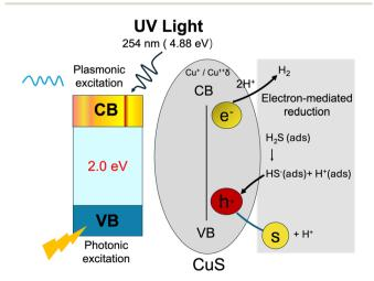
Fig. 11 Schematic illustration of the photocatalytic and plasmon-assisted decomposition of  $\rm H_2S$  over CuS under UV illumination.
