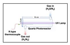
Fig. 2 Hollow jacketed quartz photoreactor for H<sub>2</sub>S photolysis.
