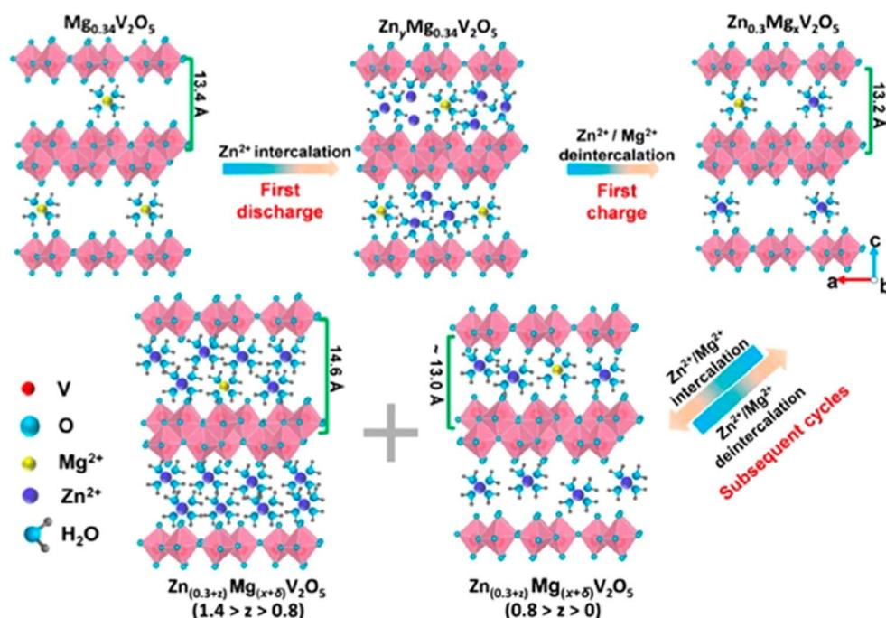
Fig. 20 Schematic illustration of the pre-intercalation of  $\text{Mg}^{2+}$  ions into  $\text{V}_2\text{O}_5$  structure, demonstrating how  $\text{Mg}^{2+}$  ions increase interlayer spacing and improve ion diffusion channels.<sup>177</sup>
