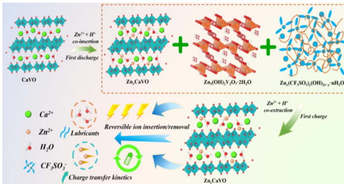
Fig. 19 Diagram illustrating the pre-intercalation of  $\text{Ca}^{2+}$  ions into the  $\text{V}_2\text{O}_5$  structure, showing how  $\text{Ca}^{2+}$  ions expand the interlayer spacing and enhance ion transport pathways.<sup>176</sup>
