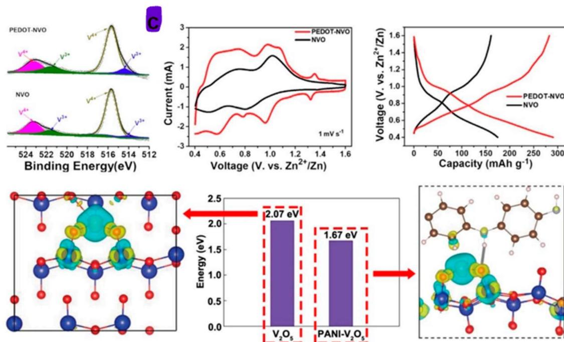
Fig. 22 The electrochemical performance evaluation of polyaniline (PANI) pre-intercalated  $V_2O_5$  as a cathode material.<sup>191</sup>
