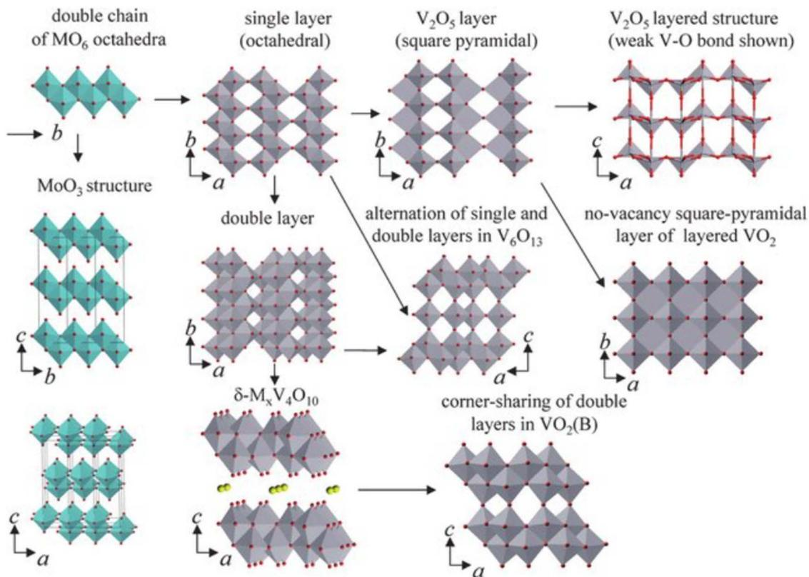
Fig. 24 Different structural forms of molybdenum-doped vanadium pentoxide ( $V_2O_5$ ).<sup>235</sup>
