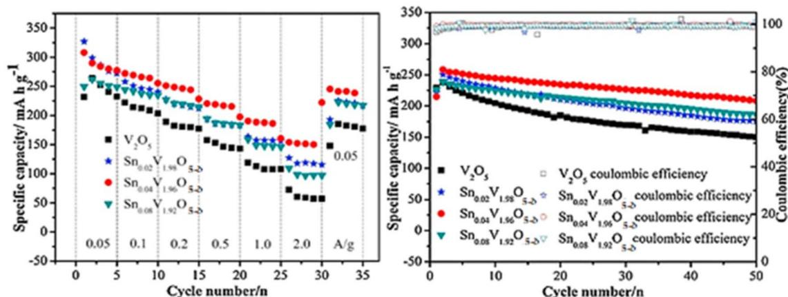
Fig. 13 Rate tests and cycling performance of electrodes at  $200 \text{ mA h g}^{-1}$ .<sup>117</sup>
