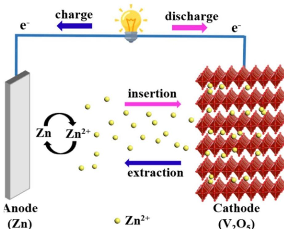
Fig. 9 Schematic illustration of the electrochemical behaviour of  $\text{Zn}/\text{V}_2\text{O}_5$  system during operation.<sup>82</sup>
