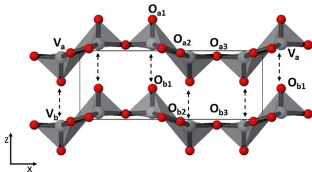
Fig. 3 Schematic structure of  $V_2O_5$  along  $c$  axis.<sup>62</sup>
