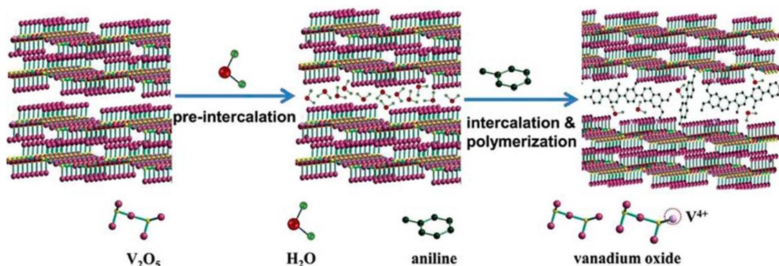
Fig. 21 Schematic diagram of the polyaniline pre-intercalated  $V_2O_5$  composite synthesis.<sup>190,191</sup>
