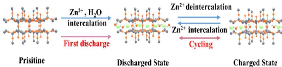
Fig. 8 Schematic illustration of  $\text{Zn}^{2+}$  and water co-intercalation into  $\text{V}_2\text{O}_5$ .<sup>81</sup>
