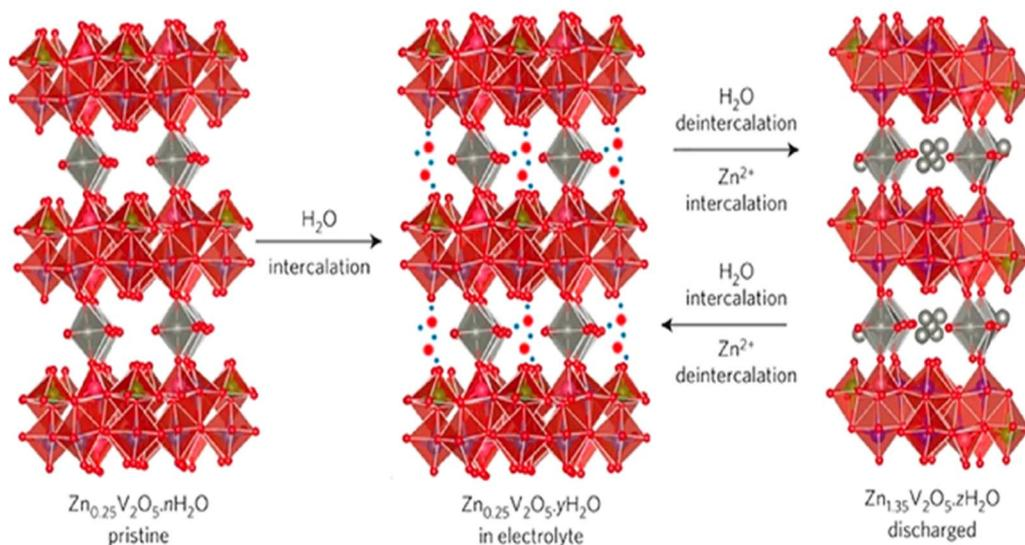
Fig. 17 Co-intercalation of  $\text{Zn}^{2+}$  cations and water molecules into the  $\text{V}_2\text{O}_5$  structure, illustrating the simultaneous insertion of both ions and water molecules.<sup>79</sup>
