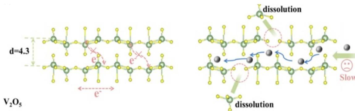
Fig. 10 The intercalation process can lead to the dissolution of the  $\text{V}_2\text{O}_5$  cathode, primarily due to the large size of the intercalating cations [ $\text{Zn}^{2+}$ ].<sup>87</sup>
