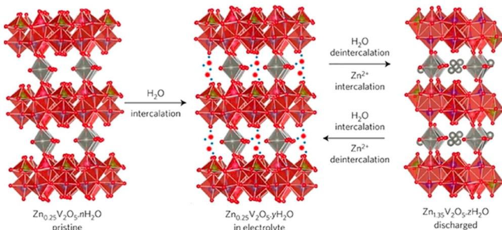
Fig. 7 Schematic of the water intercalation into  $\text{Zn}_{0.25}\text{V}_2\text{O}_5 \cdot n\text{H}_2\text{O}$  upon being immersed in aqueous electrolytes and the simultaneous  $\text{Zn}^{2+}$  intercalation–deintercalation and water deintercalation upon cycling.<sup>79</sup>
