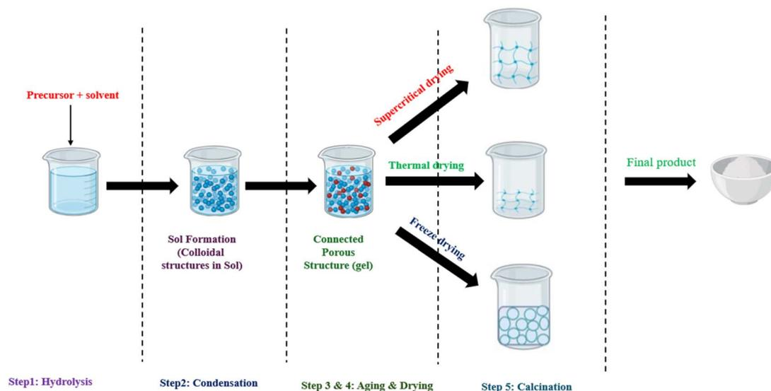
Fig. 14 Process diagram and overview of the sol-gel technique for material synthesis.
