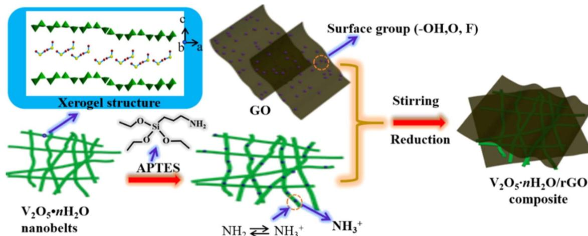
Fig. 23 Schematic diagram, illustrating the surface coating modification of  $V_2O_5$  using graphene oxide (GO).<sup>226</sup>
