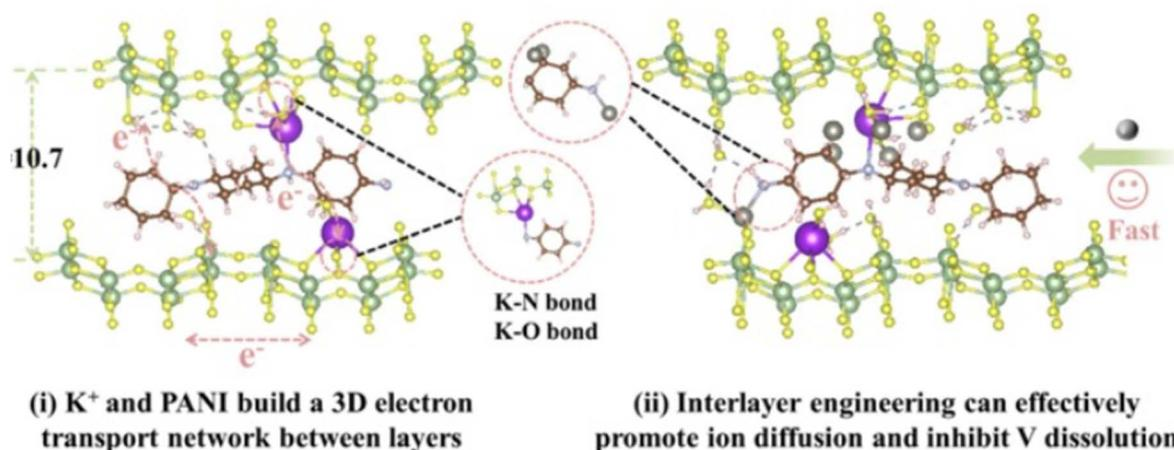
Fig. 11 Pre-intercalation technique using to enhance the electrochemical performance of  $V_2O_5$  by expanding the interlayer spacing and improving ion diffusion pathways.<sup>87</sup>
