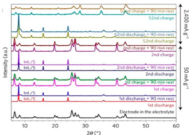
Fig. 18 XRD patterns of  $\text{Zn}_{0.25}\text{V}_2\text{O}_5 \cdot n\text{H}_2\text{O}$  at various stages of electrochemical cycling.<sup>79</sup>
