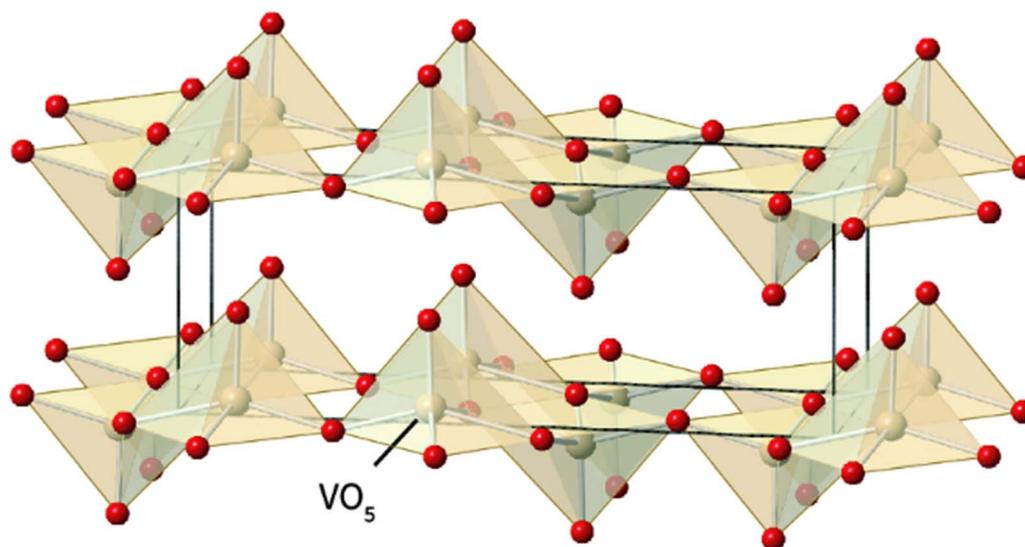
Fig. 5 The structure of vanadium oxide consists of interconnected  $\text{VO}_5$  square pyramidal units.<sup>68</sup>
