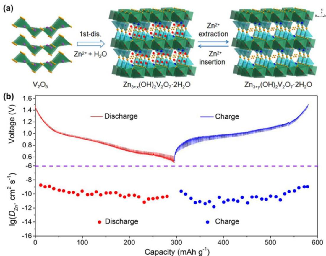
Fig. 12 (a) Co-intercalation reaction mechanism involving  $\text{Zn}^{2+}$  ions and water molecules, illustrating their simultaneous insertion into  $\text{V}_2\text{O}_5$  structure.<sup>108</sup> (b) Voltage profile of  $\text{V}_2\text{O}_5$ , showing the electrochemical behaviour during charge and discharge cycles.<sup>108</sup>
