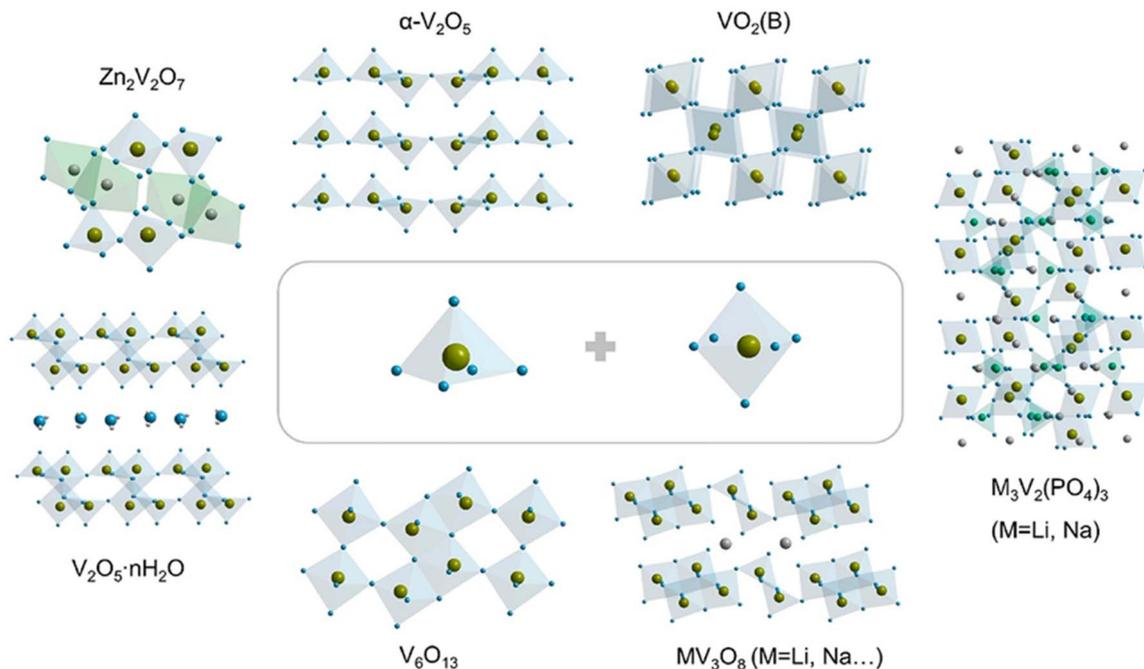
Fig. 2 Crystal structure of typical vanadium oxides: orthorhombic  $\alpha$ - $V_2O_5$ ; monoclinic  $VO_2(B)$ ,  $V_2O_5 \cdot nH_2O$ , and  $MV_3O_8$  ( $M = Li, Na, K, \dots$ ); trigonal  $V_6O_{13}$  and  $M_3V_2(PO_4)_3$  ( $M = Li, Na, K, \dots$ ); and triclinic  $Zn_2V_2O_7$ .<sup>18</sup>
