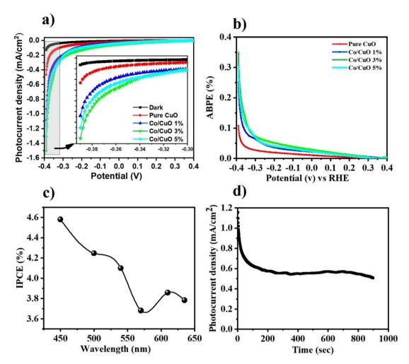
Fig. 6 PEC properties of pure CuO and Co/CuO photoelectrodes in 0.3 M  $Na_2SO_4$  as an electrolyte. (a)  $J_{ph}-V$  curves of all photocathodes, (b) ABPE% of all samples under white light illumination, (c) different values of IPCE% as a function of wavelengths for all films, and (d) the stability of the 3% Co/CuO photoelectrode under light illumination at an applied voltage of -0.4 V vs. RHE in a 0.3 M  $Na_2SO_4$  electrolyte.
