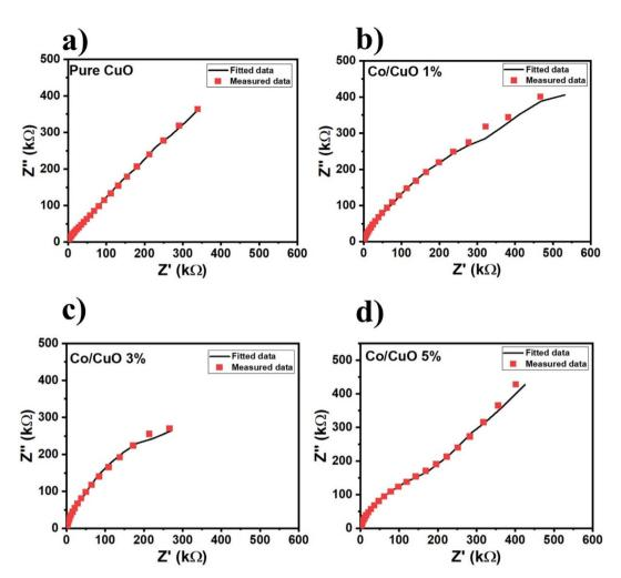
Fig. 7 EIS measurements at room temperature at 0 V vs. RHE and frequency ranges 1 mHz to 1 MHz and under white light illumination.
