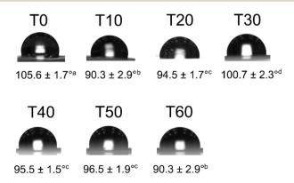
Fig. 5 Water droplets on the cross-linked chitosan film surfaces. Superscript letters represent significant differences (p < 0.05) among the samples tested under the same conditions
