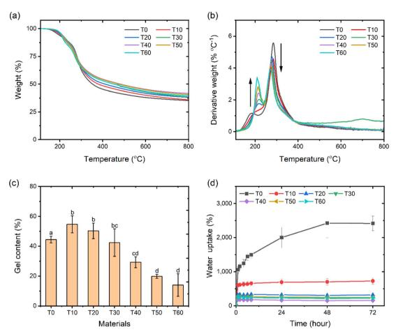
Fig. 4 Thermal stabilities of the cross-linked chitosan films with tannic acid: (a) thermogravimetric (TG) and (b) derivative TG (DTG) curves; (c) gel contents and (d) water uptakes of the chitosan films with different tannic acid loadings. Superscript letters represent significant differences ( $\rho$  < 0.05) among the samples tested under the same conditions.
