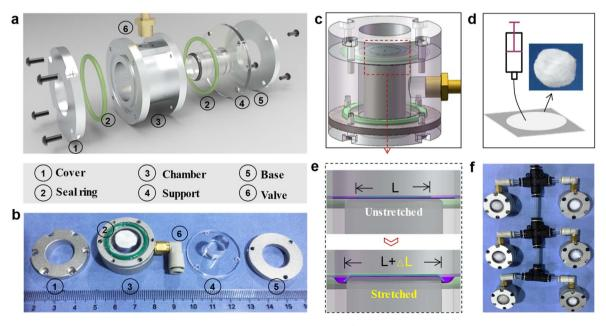
Fig. 3 (a) Dynamic stretching apparatus. (b) Components of stretching apparatus. (c) Assembled stretching unit (d) circular fibrous mat prepared from ES for piezoelectric testing. (e) Schematic illustration of the testing mechanism. (f) Assembled testing device with 6 parallel units.
