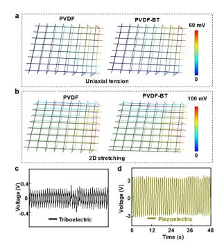
Fig. 4 Piezoelectric output. (a) Simulation of piezoelectric outputs of PVDF and PVDF-BT nanofiber under uniaxial tension and (b) 2D stretching. (c) Triboelectric and (d) Piezoelectric outputs of PVDF-BT NFMs tested with Keithley 6514.
