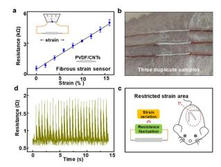
Fig. 1 Strain analysis of the rat skin. (a) Linearly resistance change of the fibrous strips as the strain increased. (b) Three strips stuck on the skin for strain detection. (c) Different directional testing of epidermal strains of rat skin. (d) Variations in the resistance of fibrous strips under normal daily conditions in rats.
