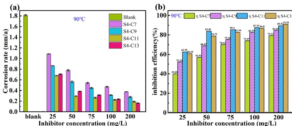
Fig. 3 Corrosion inhibition efficiency and carbon steel corrosion rate at different inhibitor concentrations in CO<sub>2</sub> systems.
