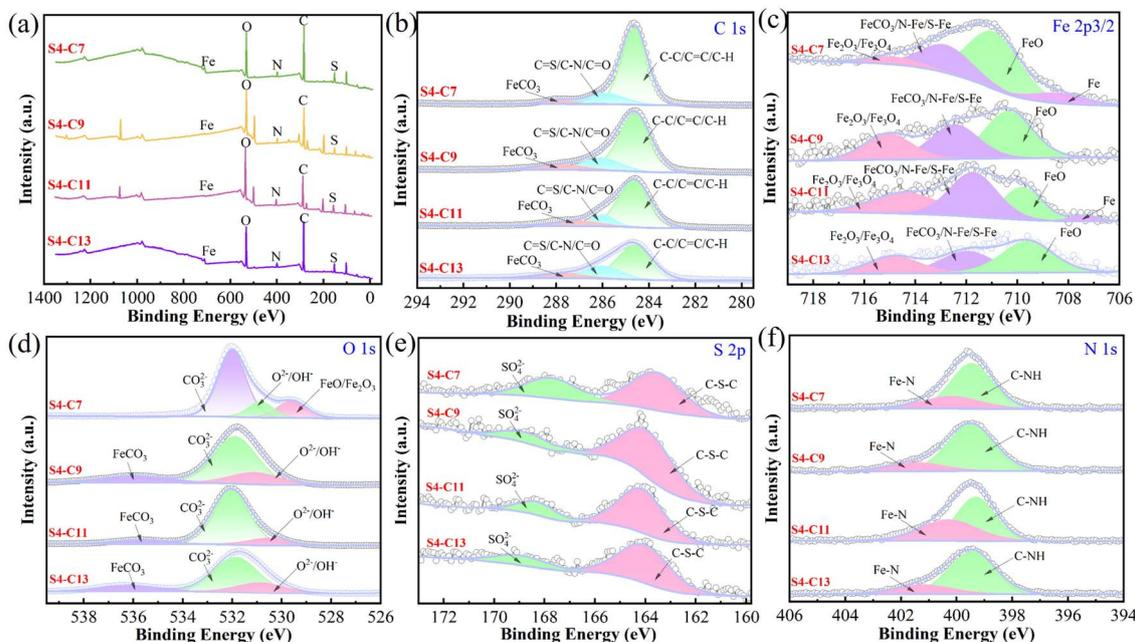
Fig. 12 Surface XPS test results of carbon steel soaked in 100 mg per L corrosion inhibitor solution at 90 °C for 22 h (a) general spectrum (b) Fe 2p<sub>3/2</sub> spectrum (c) O spectrum (d) C spectrum (e) S spectrum (f) N spectrum.
