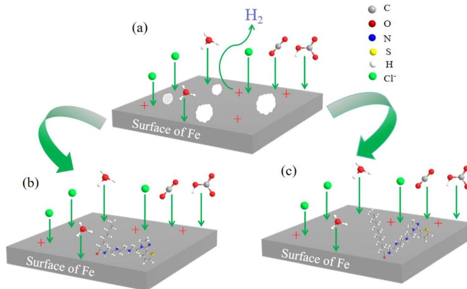
Fig. 19 Corrosion inhibition mechanism of corrosion inhibitor in CO<sub>2</sub> environment (a) blank (b) S4-C7 (c) S4-C11.
