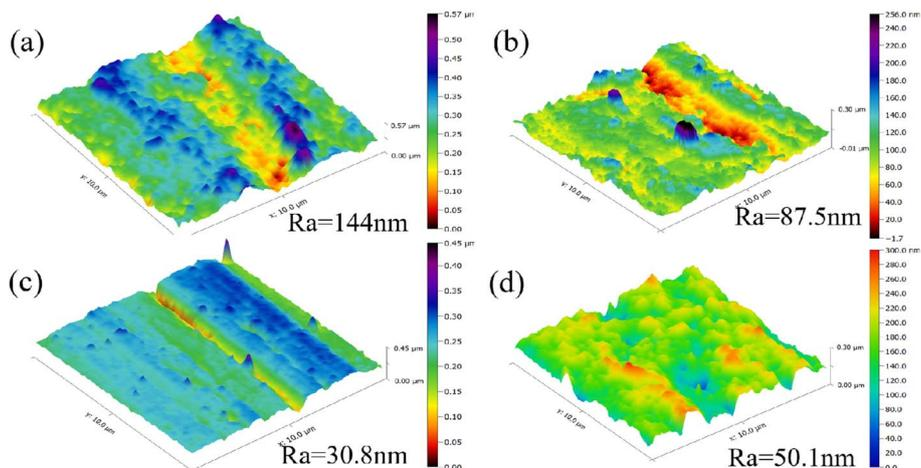
Fig. 10 Surface roughness analysis of carbon steel after corrosion for 22 h in a solution without or containing 100 mg per L imidazoline derivatives at 90 °C (a) S4-C7; (b) S4-C9; (c) S4-C11; (d) S4-C13.
