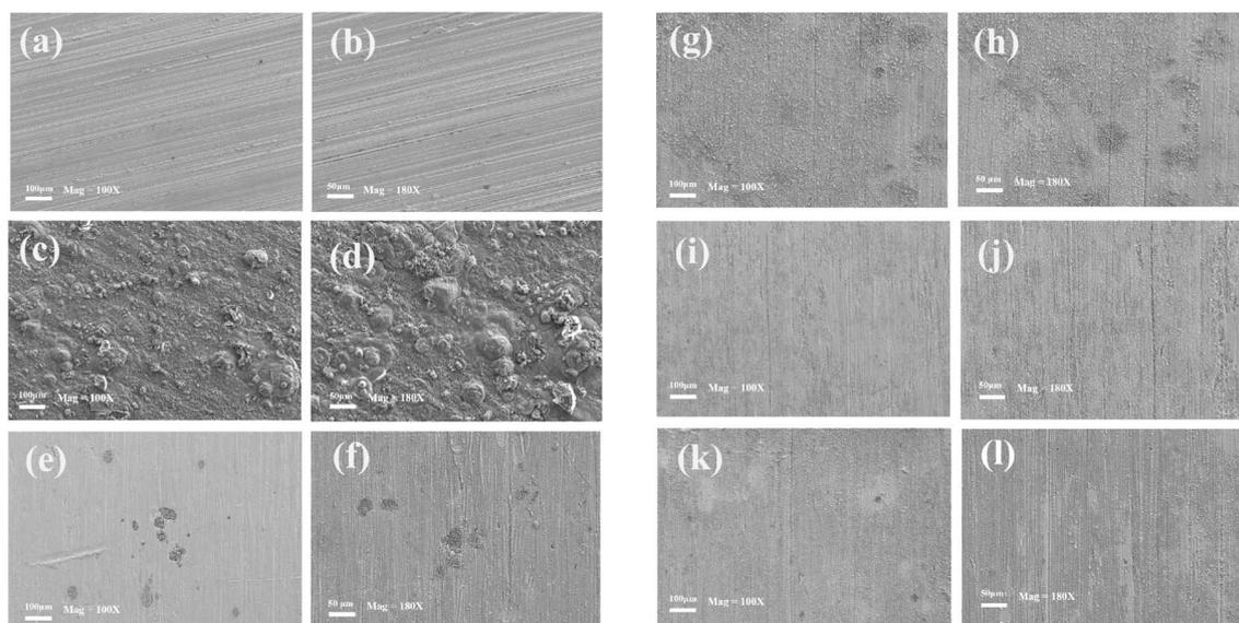
Fig. 9 Surface morphology analysis of carbon steel after corrosion for 22 h at  $90^\circ\text{C}$  in solution without or containing  $100 \text{ mg per L}$  imidazoline derivatives (SEM) (a and b) uncorroded carbon steel; (c and d) blank; (e and f) S4-C7; (g and h) S4-C9; (i and j) S4-C11; (k and l) S4-C13.
