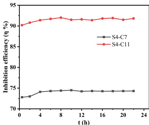
Fig. 8 Time dependence of inhibition efficiency of S4-C11 and S4-C7 (100 mg mL<sup>-1</sup>) for Q235 carbon steel in CO<sub>2</sub>-saturated oilfield produced water at 90 °C.
