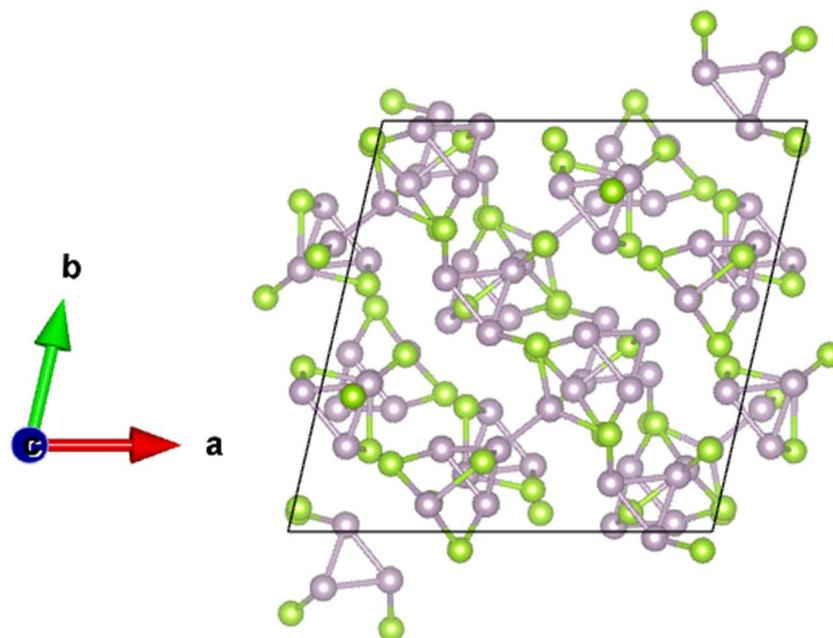
Fig. 4 The optimized structure of slab-(110) of  $P_4Se_3$ .
