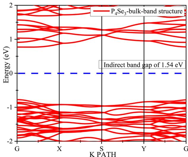
Fig. 7 The electronic band diagram for bulk  $P_4Se_3$ , where the Fermi level was set at 0 eV.
