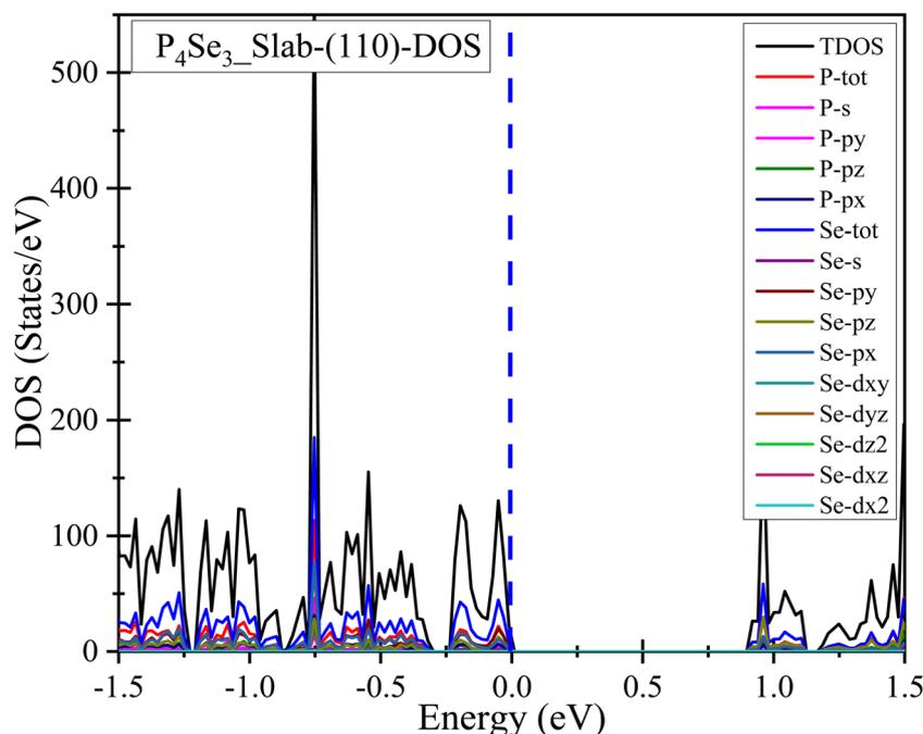
Fig. 11 The electronic partial and total DOS for slab-(110) of  $P_4Se_3$ .
