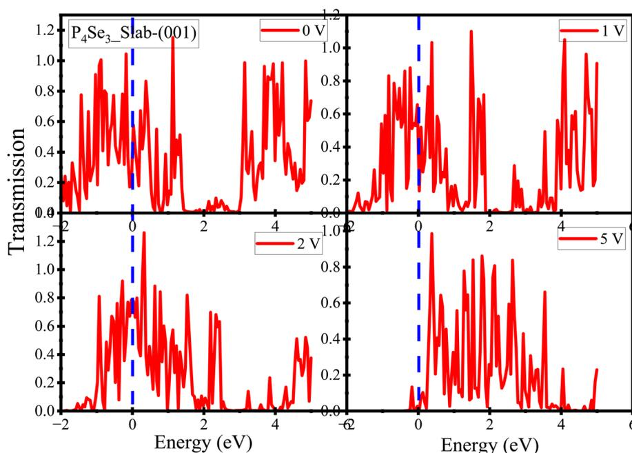
Fig. 15 The transmission spectra for slab-(001) of  $P_4Se_3$  in the range 0–5 V.
