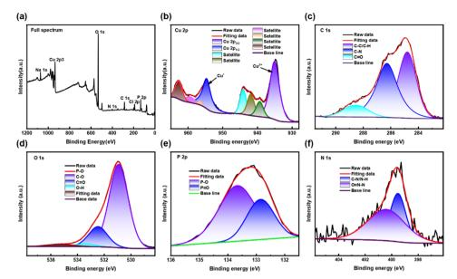
Fig. 3 XPS spectral deconvolution of Lac-NFs: (a) survey scan confirming elemental composition, with high-resolution spectra of (b) Cu<sup>2+</sup> 2p<sub>3/</sub> 2-2p<sub>1/2</sub> orbitals, (c) C 1s revealing C-C/C-O bonds, (d) O 1s showing metal-oxygen coordination, (e) P 2p phosphate signatures, and (f) N 1s amide linkages characteristic of enzyme integration.
