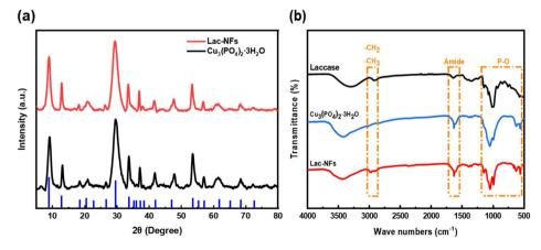
Fig. 4 XRD patterns and FT-IR spectra of Lac-NFs. (a) XRD patterns of La-NFs  $versus Cu_3(PO_4)_2 \cdot 3H_2O$  demonstrating hybrid structure formation. (b) FT-IR spectra of La-NFs, Cu<sub>3</sub>(PO<sub>4</sub>)<sub>2</sub>·3H<sub>2</sub>O, and free laccase confirming successful enzyme immobilization through interfacial interactions.
