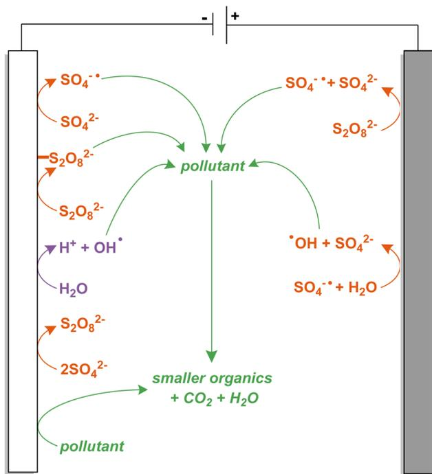
Fig. 1 Electrochemically activated persulphate.
