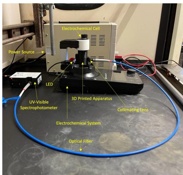
Fig. 2 Real-time *in situ* continuous monitoring apparatus (48 × 61 × 20 cm).
