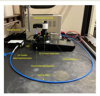
Fig. 2 Real-time in situ continuous monitoring apparatus (48  $\times$  61  $\times$  20 cm).
