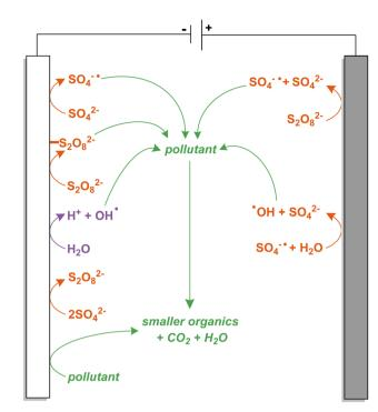
Fig. 1 Electrochemically activated persulphate.
