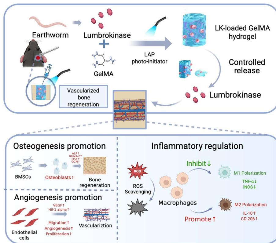
**Scheme 1** Schematic diagram illustrating the constitution of the LK-loaded GelMA hydrogel and its LK sustained-release for bone defect repair by enhancing angiogenesis, osteogenesis, and inflammatory regulation.
