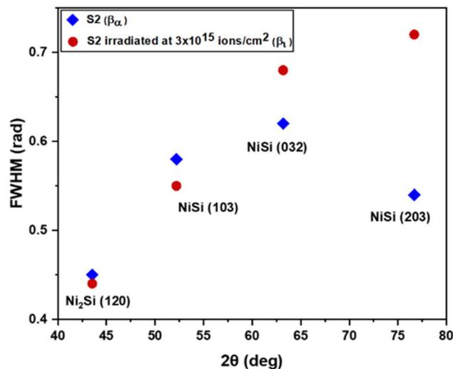
Fig. 4 FWHM comparison of nickel silicide phases; Ni<sub>2</sub>Si(120), NiSi(103), NiSi(032) and NiSi(203), in annealed bilayer sample and sample irradiated post annealing.
