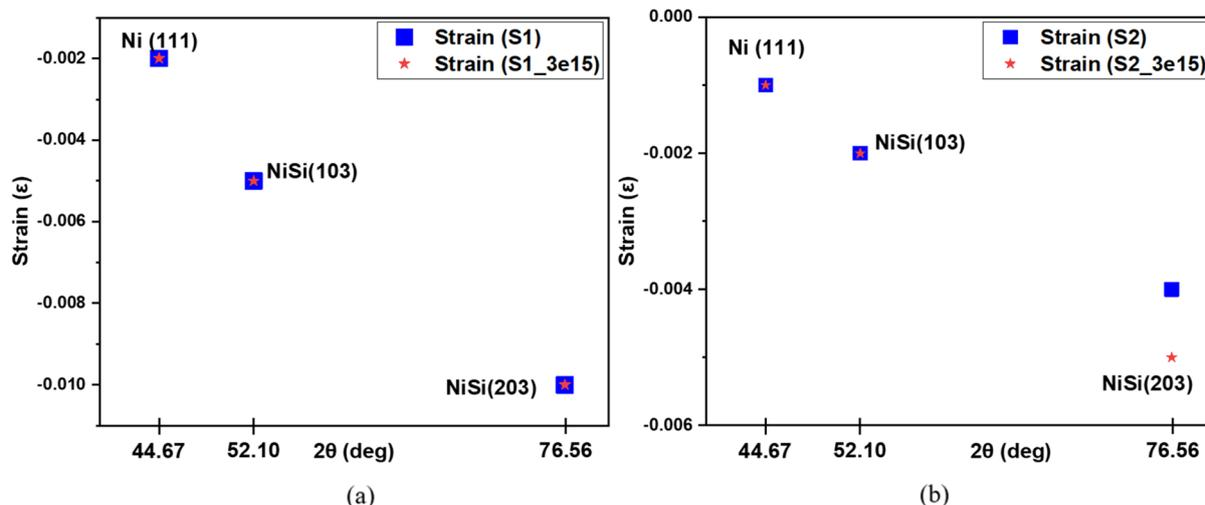
Fig. 5 Strain in (a) as deposited and irradiated samples, and (b) annealed and irradiated post annealing sample in phases Ni (111), NiSi (103) and NiSi (203). The annealing value taken is  $3 \times 10^{15}$  ions per  $\text{cm}^2$ .
