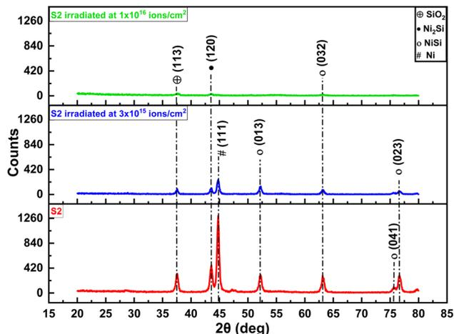
Fig. 3 The GIXRD diffractogram in the figure shows the phases of nickel silicides  $\text{Ni}_2\text{Si}$  and  $\text{NiSi}$  of different orientation in the annealed sample and samples irradiated post annealing under fluence  $3 \times 10^{15}$  ions per  $\text{cm}^2$   $1 \times 10^{16}$  ions per  $\text{cm}^2$ . The decrease in peak intensities of the phases is clearly visible as the fluence increases indicating progressive amorphization of these silicide phases.
