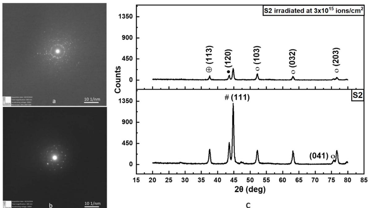
Fig. 7 SAED pattern for (a) annealed sample, (b) irradiated with  $3 \times 10^{15}$  ions per  $\text{cm}^2$  post annealing sample, (c) diffractogram comparison of annealed sample and irradiated post annealing sample.
