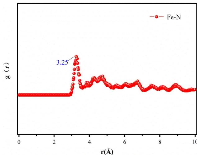
**Fig. 15** RDF of  $[C_{12}\text{Py}]\text{Br}$  adsorption on Fe(110) surface.
