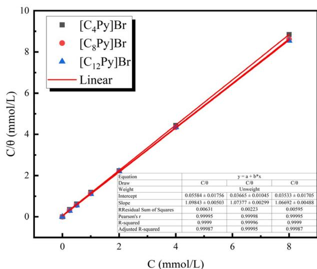
Fig. 9 Langmuir adsorption plot of [C<sub>n</sub>Py]Br ILs for mild steel in 1 M HCl.
