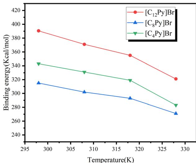
**Fig. 14** Calculation of adsorption energy of  $[C_{12}\text{Py}]\text{Br}$  ILs on Fe(110) surface in aqueous HCl solution at different temperatures.
