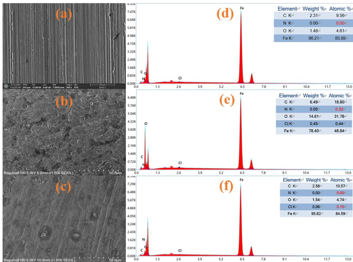
Fig. 10 SEM images and corresponding EDS spectra are shown for (a and d) mild steel prior immersion in HCl, (b and e) after 24 h of immersion in HCl without the inhibitor, (c and f) with  $[C_{12}Py]Br$ .
