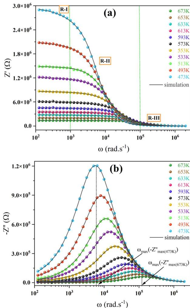
**Fig. 6** (a) Variation of real part of the impedance with angular frequency at various temperatures for NaCdP<sub>3</sub>O<sub>9</sub>. (b) Variation of imaginary part of the impedance with angular frequency at various temperatures for NaCdP<sub>3</sub>O<sub>9</sub>.
