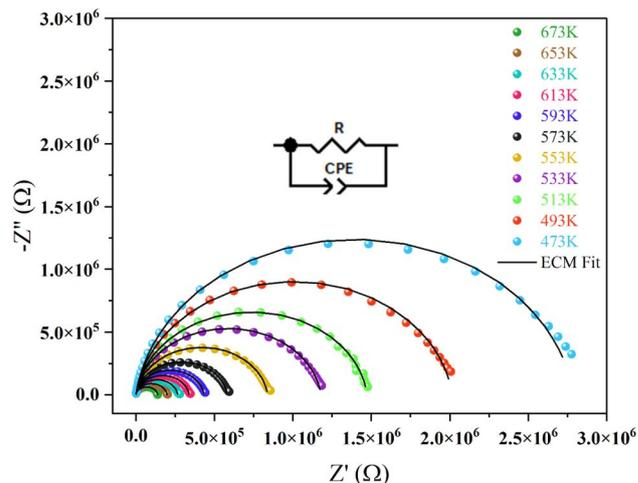
Fig. 5 Nyquist plot of NaCdP<sub>3</sub>O<sub>9</sub> compound, at different temperatures with equivalent circuit model in the inset.
