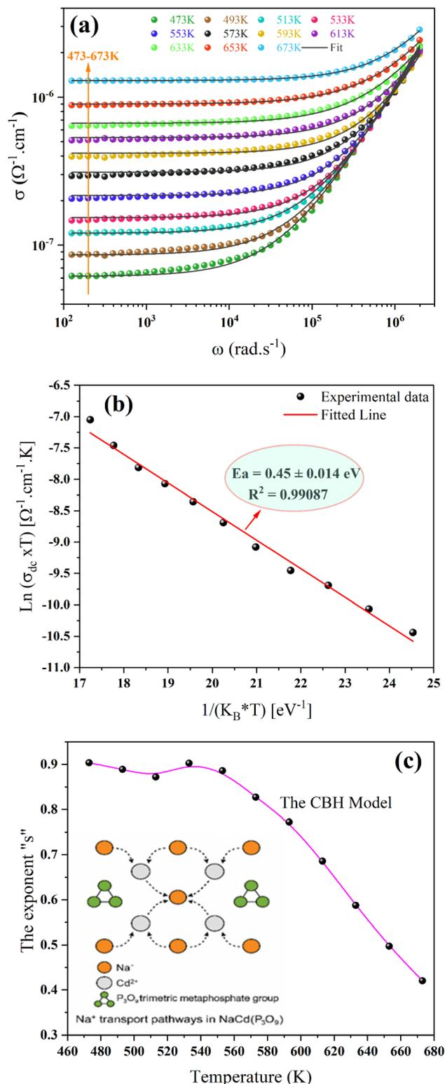
Fig. 7 (a) Frequency-dependent variation of the electrical conductivity of NaCdP<sub>3</sub>O<sub>9</sub> at different temperatures. (b) Evolution of  $\ln(\sigma_{dc} \times T)$  versus the reciprocal of temperature and the deduced activation energy value. (c) The temperature dependence of the frequency exponent "s".
