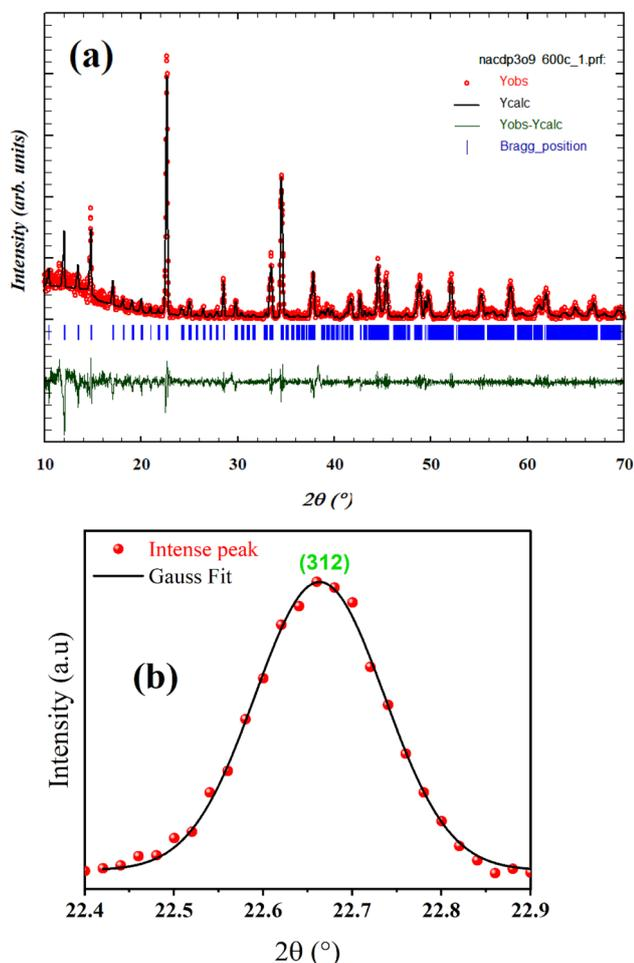
Fig. 2 (a) X-ray diffraction (XRD) of NaCdP<sub>3</sub>O<sub>9</sub> at room temperature. (b) The Debye–Scherrer plot for NaCdP<sub>3</sub>O<sub>9</sub> compound.
