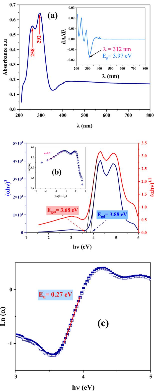
Fig. 4 (a) The UV-vis absorbance spectrum and  $dA/d\lambda$  as a function of  $\lambda$  (inset) for the phosphors NaCdP<sub>3</sub>O<sub>9</sub>. (b) Variation of  $(\alpha h\nu)^2$  and  $(\alpha h\nu)^{1/2}$  plots vs.  $h\nu$  for band gap of NaCdP<sub>3</sub>O<sub>9</sub> and variation of  $\ln(\alpha h\nu)$  against  $\ln(h\nu - E_g)$  determination (inset). (c) Determining the Urbach energy.
