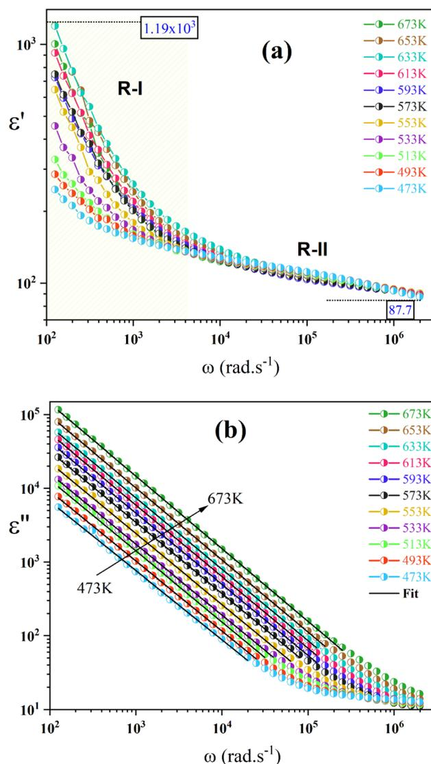
Fig. 9 (a) Evolution of the real part of the permittivity as a function of the angular frequency of the NaCdP<sub>3</sub>O<sub>9</sub> at various temperatures. (b) Evolution of the imaginary part of the permittivity as a function of the angular frequency of the NaCdP<sub>3</sub>O<sub>9</sub> at various temperatures.
