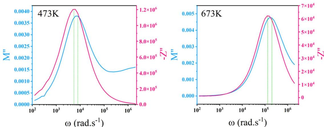
Fig. 13 Combined  $Z''$  and  $M''$  spectroscopic plots.
