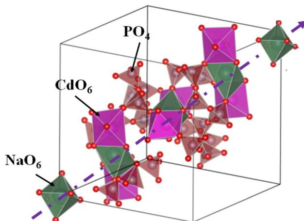
Fig. 8 Sodium-ion diffusion pathway in the NaCdP<sub>3</sub>O<sub>9</sub> structure along the [111] direction.
