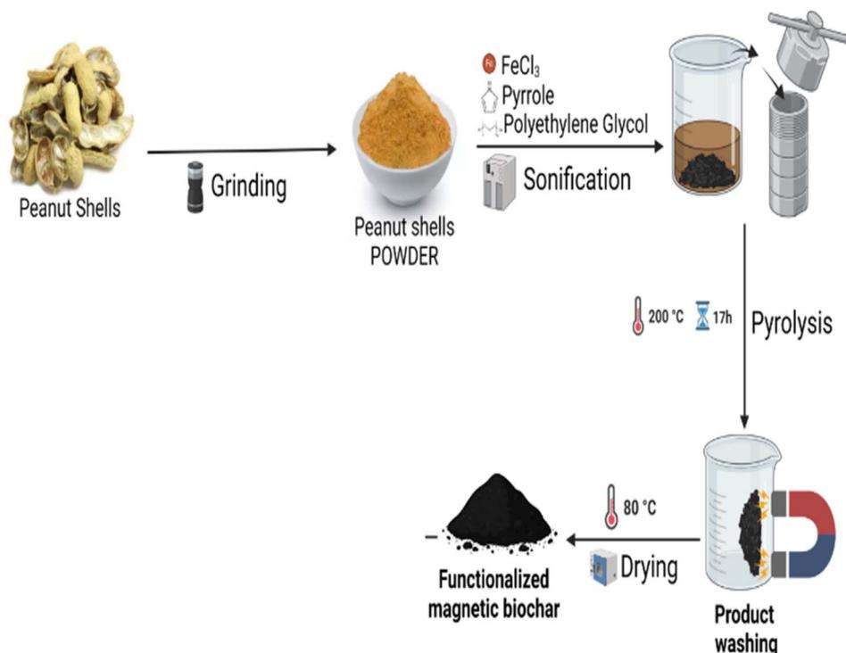
Fig. 1 Synthesis of Pyrrole Functionalized Magnetic Biochar (PFMB) nanocomposite (reproduced from our early work<sup>14</sup>).
