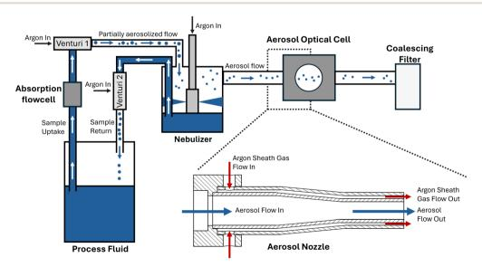
Fig. 1 Schematic overview of the liquid recirculating system used for spectroscopic characterization of aqueous process fluids in this work.<sup>38</sup> Fluid flows are shown with arrows. Zoomed-in regions shows aerosol flow directed by a nozzle into the optical cell.
