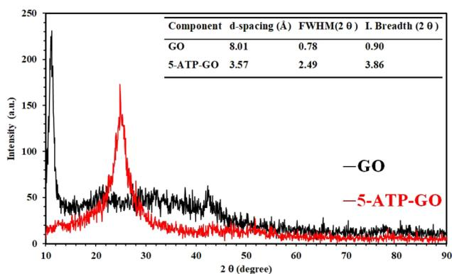
Fig. 4 XRD diffractograms of GO and 5-ATP-GO.
