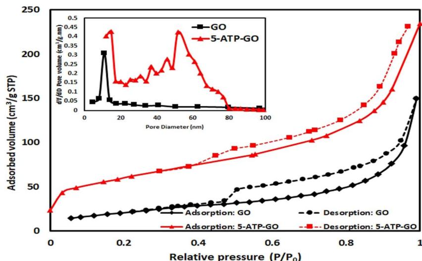
Fig. 8 BET analysis and pore diameter distribution of GO and 5-ATP-GO.
