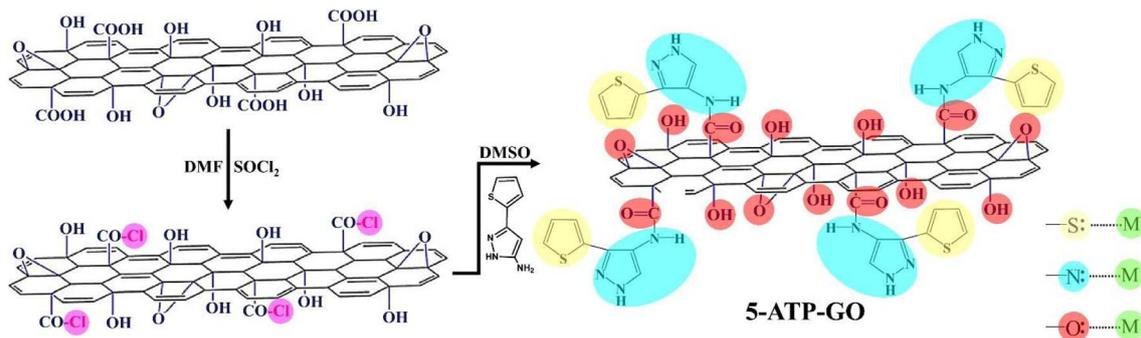
Fig. 1 Scheme of GO modification by 5-amino-3(2-thienyl) pyrazole.
