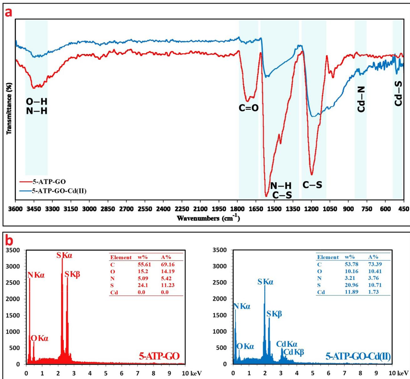
Fig. 17 (a) FTIR spectra and (b) EDX analysis of 5-ATP-GO before and after cadmium adsorption.
