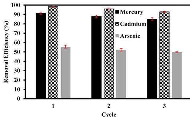
Fig. 18 The number of adsorption–desorption cycles of Cd(II) Hg(II), and As(III) on 5-ATO-GO at 1.0 M HCl concentration.
