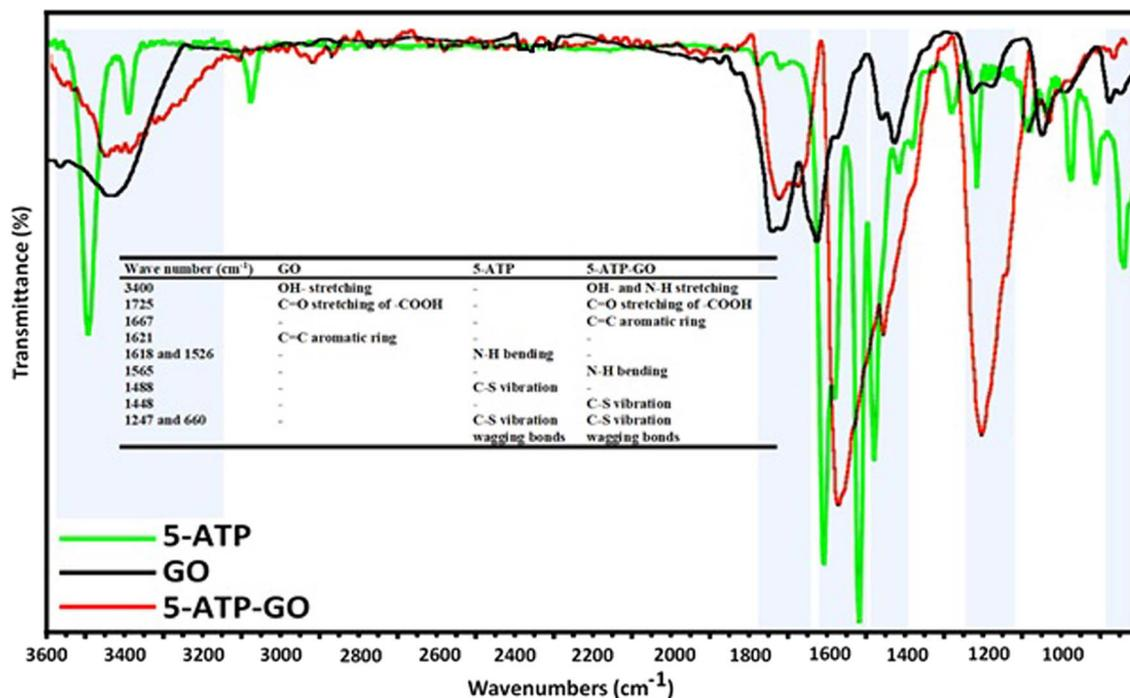
Fig. 2 FTIR spectra of GO and 5-ATP-GO composites.
