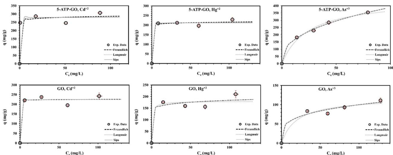
Fig. 16 Representation of the Langmuir, Freundlich, and Sips isotherm models for GO and 5-ATP-GO in nonlinear regression analysis by comparison with experimental data, for Hg(II), Cd(II), and As(III) sorption at 25 °C under optimum conditions.
