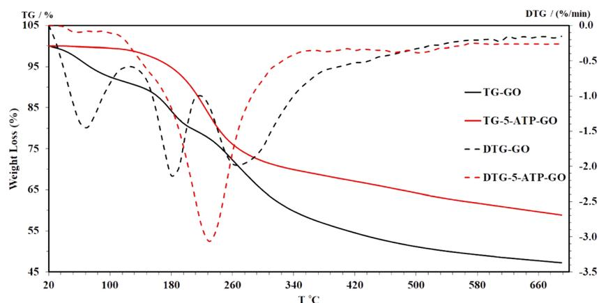
Fig. 3 Thermogravimetric and derivative thermogravimetric curves of GO and 5-ATP-GO.
