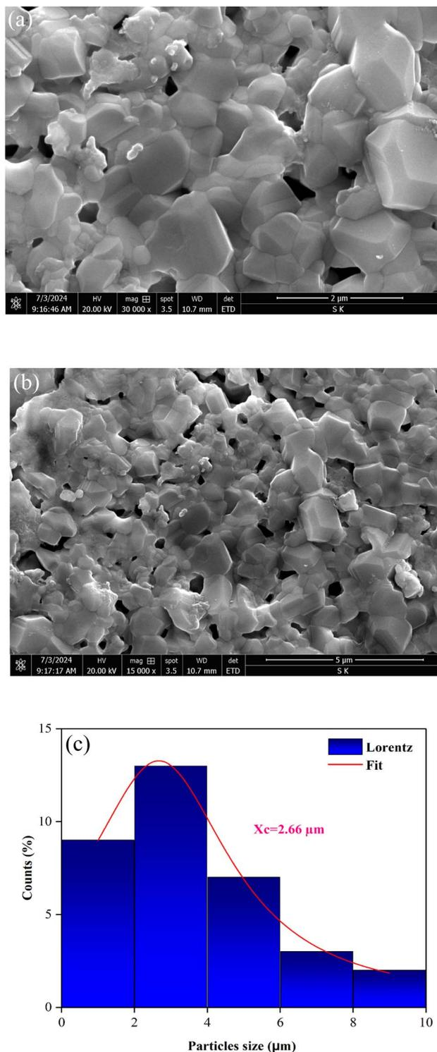
Fig. 2 (a) SEM image of  $\text{Li}_2\text{CoP}_2\text{O}_7$ . (b) SEM image of  $\text{Li}_2\text{CoP}_2\text{O}_7$ . (c): The corresponding average particle size histogram of  $\text{Li}_2\text{CoP}_2\text{O}_7$ .
