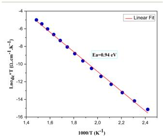
Fig. 10 Evolution of  $\ln(\sigma_{dc} \times T)$  as a function of (1000/T).
