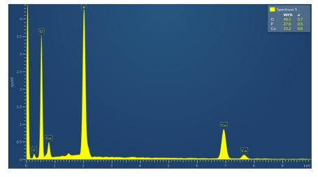
Fig. 3 EDX spectrum of the fractured surface of Li<sub>2</sub>CoP<sub>2</sub>O<sub>7</sub>.
