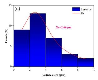
Fig. 2 (a) SEM image of Li<sub>2</sub>CoP<sub>2</sub>O<sub>7</sub>. (b) SEM image of Li<sub>2</sub>CoP<sub>2</sub>O<sub>7</sub>. (c): The corresponding average particle size histogram of Li<sub>2</sub>CoP<sub>2</sub>O<sub>7</sub>.
