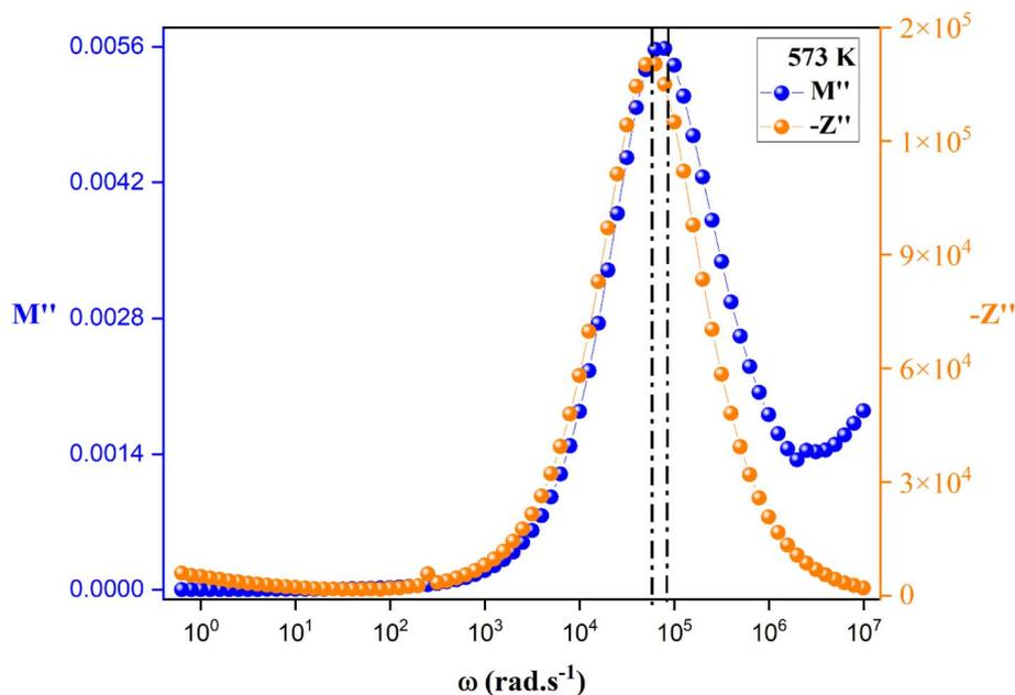
Fig. 13 Combined  $M''$  and  $-Z''$  spectroscopic plots.
