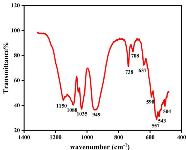
Fig. 5 The FTIR spectrum of Li<sub>2</sub>CoP<sub>2</sub>O<sub>7</sub> compound.
