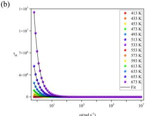
Fig. 7 (a) Frequency-dependent of real part of dielectric constants ( $\varepsilon'$ ) of Li<sub>2</sub>CoP<sub>2</sub>O<sub>7</sub>. (b) Imaginary part ( $\varepsilon''$ ), at different temperature of Li<sub>2</sub>CoP<sub>2</sub>O<sub>7</sub>.
