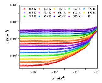
Fig. 8 The variation of  $ln(\sigma_{ac})$  versus  $ln(\omega)$  at different temperatures of Li<sub>2</sub>CoP<sub>2</sub>O<sub>7</sub>.
