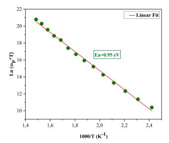
Fig. 12 Dependence of  $ln(\omega_p)$  versus reciprocal temperature for  $Li_2CoP_2O_7$ .
