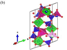
Fig. 1 (a) Rietveld refinement profile carried out through full proof software of  $\text{Li}_2\text{CoP}_2\text{O}_7$ . (b) Crystal structure of  $\text{Li}_2\text{CoP}_2\text{O}_7$ .
