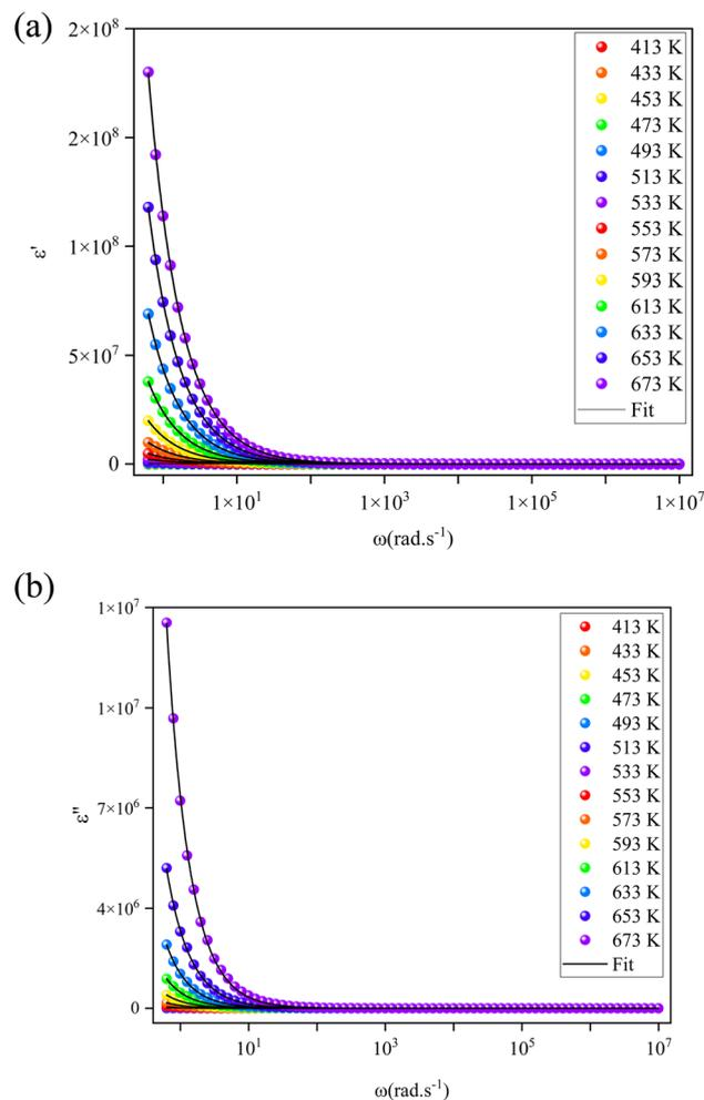
Fig. 7 (a) Frequency-dependent of real part of dielectric constants ( $\epsilon'$ ) of  $\text{Li}_2\text{CoP}_2\text{O}_7$ . (b) Imaginary part ( $\epsilon''$ ), at different temperature of  $\text{Li}_2\text{CoP}_2\text{O}_7$ .
