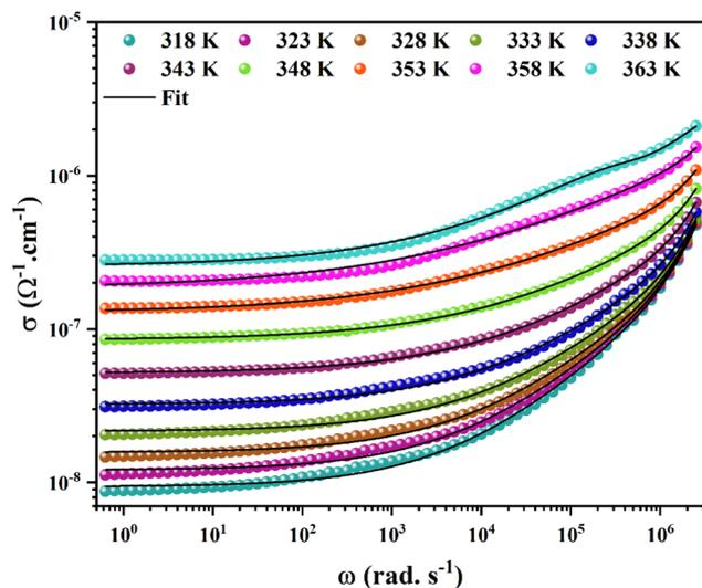
Fig. 9 Frequency dependence of ac conductivity for different temperatures.
