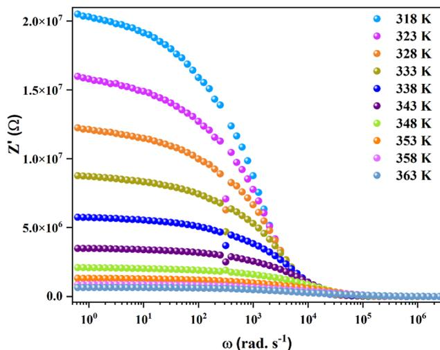
Fig. 7 Frequency dependence of  $Z'$  at various temperatures of  $(C_6H_9N_2)_3[BiBr_6] \cdot H_2O$  compound.
