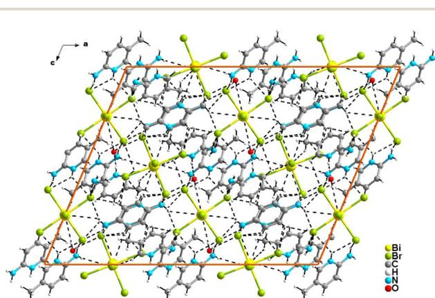
Fig. 1 Projection of the structure of (C<sub>6</sub>H<sub>9</sub>N<sub>2</sub>)<sub>3</sub>[BiBr<sub>6</sub>]·H<sub>2</sub>O along the crystallographic *b*-axis.
