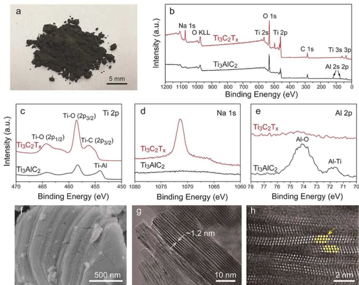
Fig. 5 (a) Digital photograph of  $Ti_3C_2T_x$  powder (b) survey XPS scan of  $Ti_3AlC_2$  MAX and  $Ti_3AlC_2$  MX (c–e) high-resolution orbital XPS scan of  $Ti_3AlC_2$  MAX and  $Ti_3AlC_2$  MX (f–h) SEM, TEM and HAADF-STEM micrographs of  $Ti_3AlC_2$  MX (reprinted with permission from John Wiley and Sons<sup>126</sup>).
