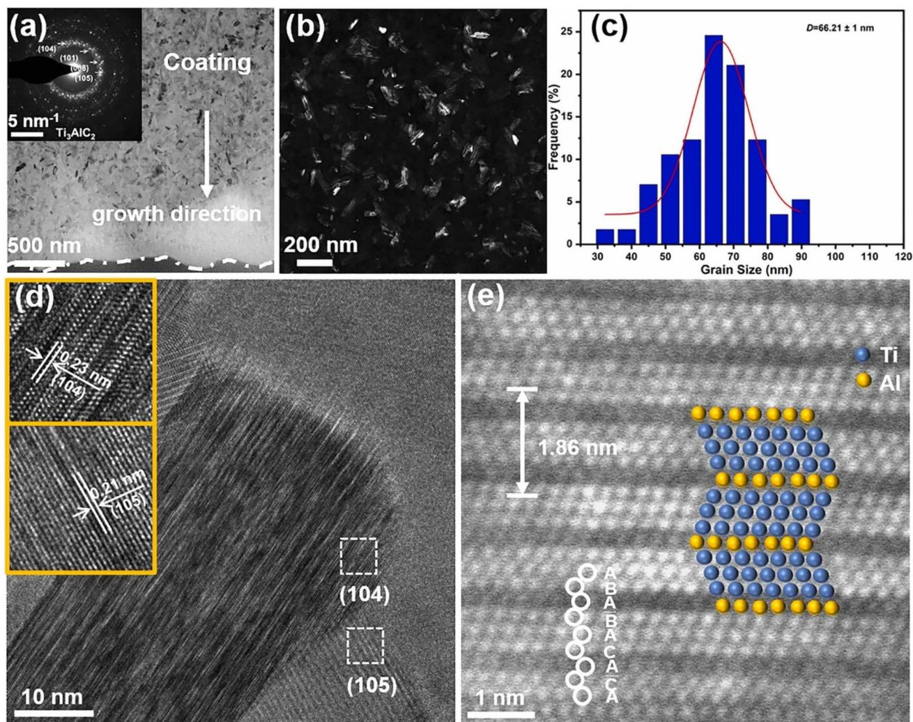
Fig. 4 (a and b) TEM micrographs of HiPIMS induced synthesis of  $\text{Ti}_3\text{AlC}_2$  MAX phase, (c) grain size distributions calculated for (b) and (d) HRTEM micrographs of  $\text{Ti}_3\text{AlC}_2$ , (e) atomic arrangement STEM micrographs of  $\text{Ti}_3\text{AlC}_2$  (reprinted with permission from Elsevier<sup>58</sup>).
