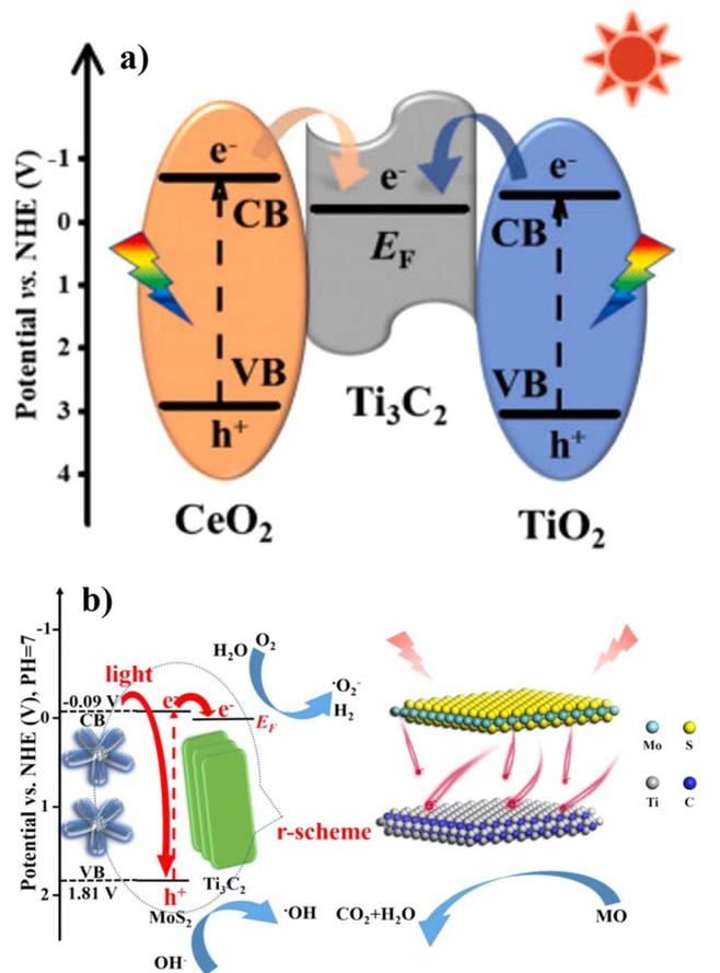
Fig. 11 Schematic representation of photocatalytic mechanism of (a) CeO<sub>2</sub>/Ti<sub>3</sub>C<sub>2</sub>/TiO<sub>2</sub> – M-scheme (b) Ti<sub>3</sub>C<sub>2</sub>/MoS<sub>2</sub> – r-scheme (reprinted with permission from Elsevier<sup>94</sup>).
