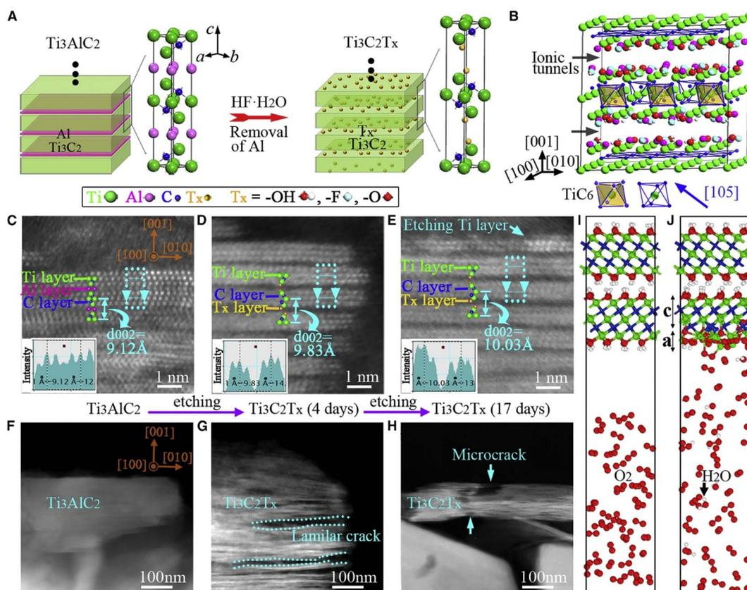
Fig. 8 (A and B) Scheme of Ti<sub>3</sub>C<sub>2</sub>T<sub>x</sub> synthesis (C–H) representation ADF micrographs of Ti<sub>3</sub>C<sub>2</sub>T<sub>x</sub> (I and J) MD simulation of Ti<sub>3</sub>C<sub>2</sub>T<sub>x</sub>.
