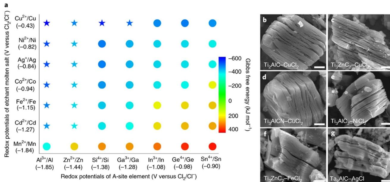
Fig. 6 (a) Redox potentials of A-sites in various MAX phases compared to molten salt (Cl<sup>-</sup>) etchants of different cations, indicated based on Gibbs free energy. (b–g) SEM micrographs of various MXenes etched from MAX phases with different A-sites and corresponding Lewis acids (reprinted with permission from *Nature Materials*<sup>127</sup>).
