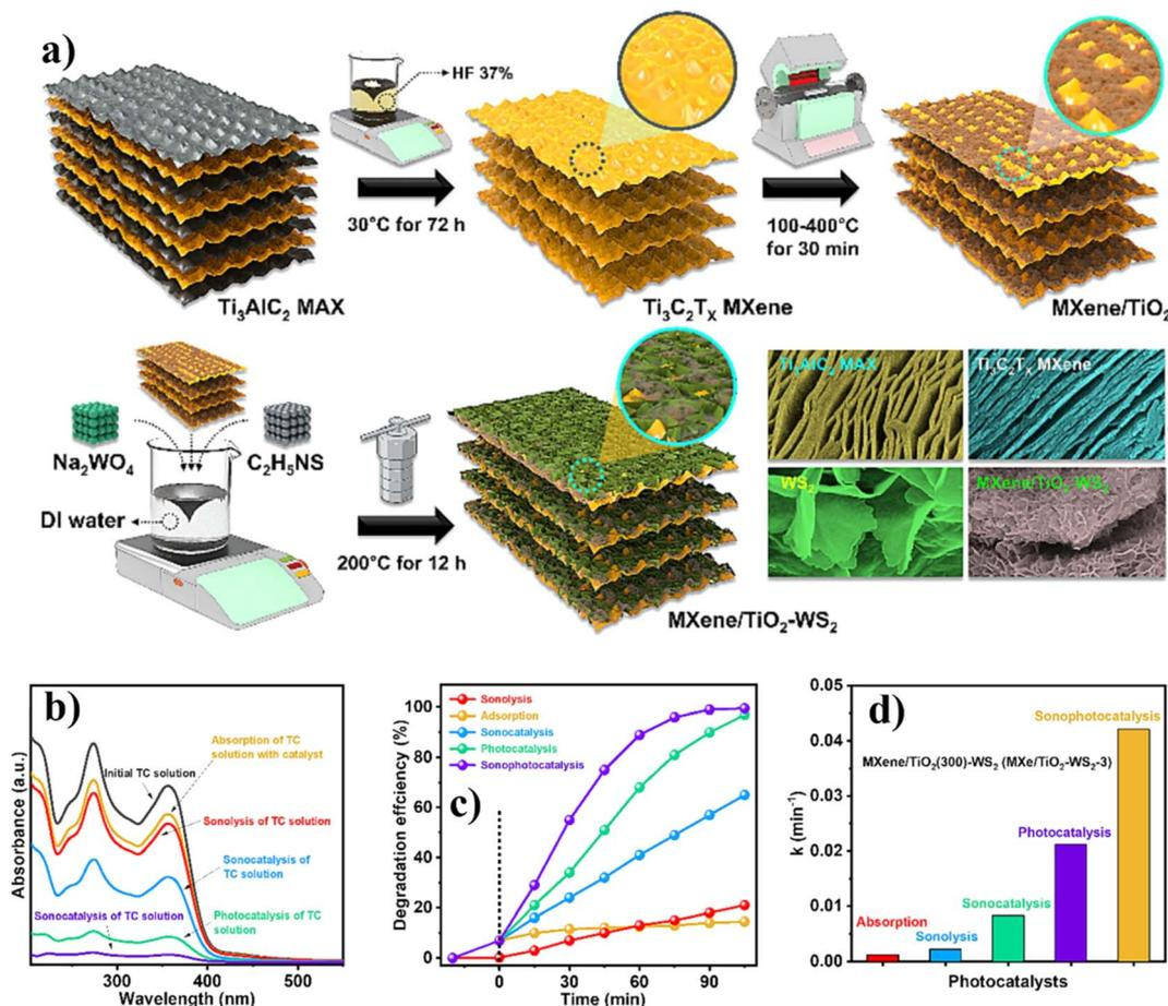
Fig. 13 (a) Schematic illustration of  $\text{Ti}_3\text{C}_2\text{T}_x\text{@TiO}_2\text{-WS}_2$  nanostructure synthesis. (b) UV-vis spectra of TC degradation under various AOP and h-AOP conditions. (c & d) Degradation efficiency and rate comparison of different AOPs using  $\text{Ti}_3\text{C}_2\text{T}_x\text{@TiO}_2\text{-WS}_2$ .
