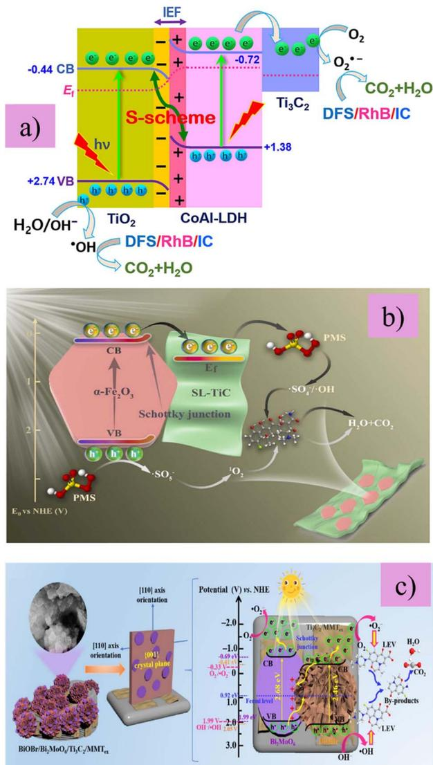
Fig. 10 Schematic representation of plausible S-scheme mechanism of photocatalytic degradation of targeted pollutants using (a) CoAl-LDH/TiO<sub>2</sub>/Ti<sub>3</sub>C<sub>2</sub> (b)  $\alpha$ -Fe<sub>2</sub>O<sub>3</sub>/Ti<sub>3</sub>C<sub>2</sub> (c) BiOBr/Bi<sub>2</sub>MoO<sub>6</sub>/Ti<sub>3</sub>C<sub>2</sub>/MMT<sub>ex</sub> (reprinted with permission from Elsevier<sup>91–93</sup>).
