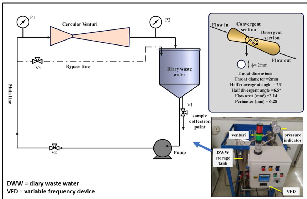
Fig. 2 HC set up and its schematic diagram along with circular venturi insight.
