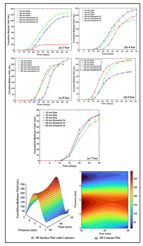
Fig. 5 Cumulative Methane yield from DWW treated by HC at different pressures: (a) 3 bar, (b) 4 bar, (c) 5 bar, (d) 6 bar, and (e) 7 bar. (f) 3D surface plot and (g) 2D contour plot.
