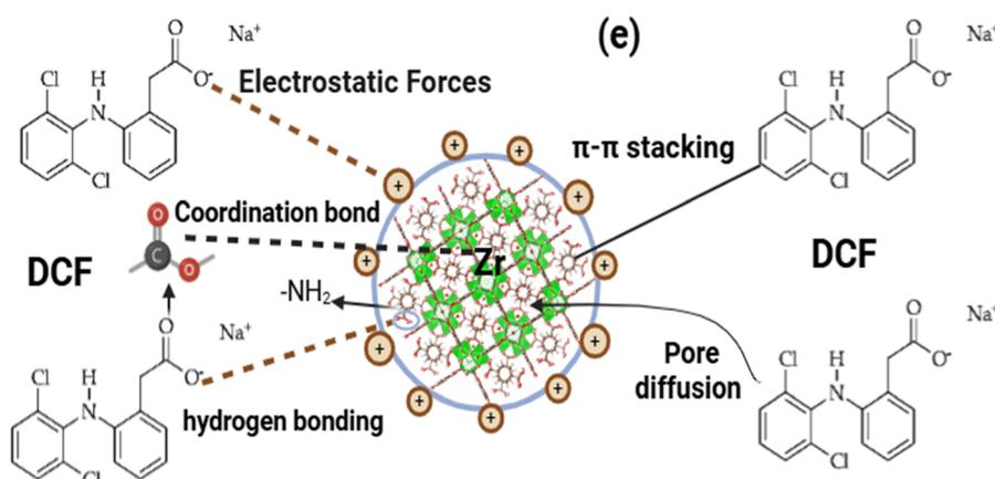
Fig. 7 (a–d) XPS analysis showing the changes in the surface composition of Zr-MOF@C after DCF adsorption; (e) proposed mechanism of the adsorption of DCF on Zr-MOF@C.
