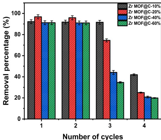
Fig. 8 Removal efficiency of Zr-MOF@C composites across multiple adsorption–desorption cycles (at 22 °C, time 24 h; pH 7; dose 10 mg; and initial concentration 30 mg L<sup>-1</sup>).
