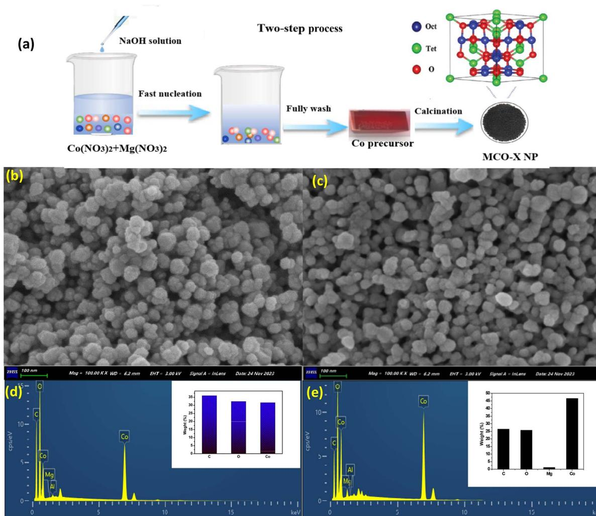
Fig. 1 (a) Schematic illustration of the preparation of MCO-X catalysts, SEM images of (b)  $\text{Co}_3\text{O}_4$  and (c) MCO-0.2; EDS spectra for (d)  $\text{Co}_3\text{O}_4$  and (e) MCO-0.2, respectively.
