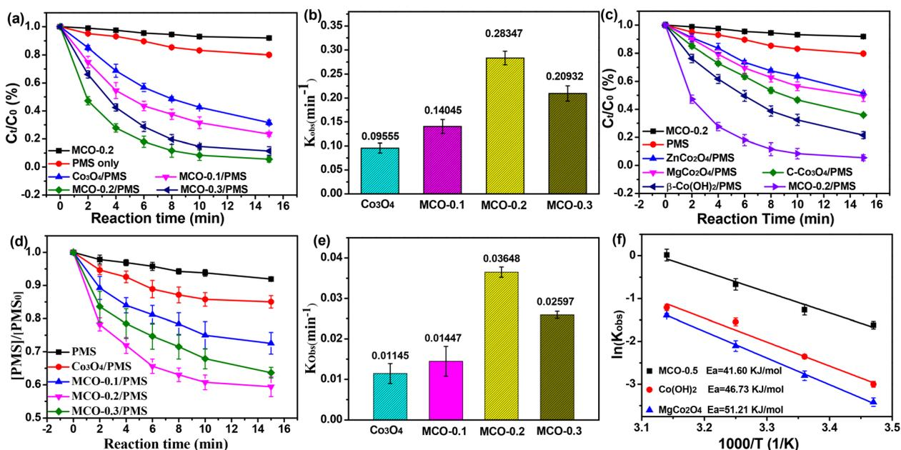
Fig. 3 (a) THIA removal and (d) PMS depletion over  $\text{Co}_3\text{O}_4$  and MCO- $X$  catalysts, (b) and (e) the corresponding first-order rate constants; (c) THIA removal curves over MCO-0.2 and other similar catalysts, (f) the corresponding Arrhenius plots. Experiment conditions:  $\text{pH} = 7$ ,  $[\text{THIA}] = 20 \text{ mg L}^{-1}$ ,  $[\text{catalyst}] = 100 \text{ mg L}^{-1}$ ,  $[\text{PMS}] = 0.4 \text{ mM}$ .
