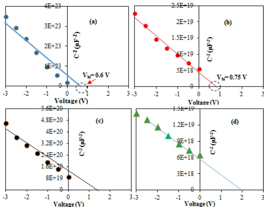
Fig. 8  $C^{-2}$ - $V$  characteristics of (a) CdS/Si heterojunction before IPL annealing, (b) CdS/Si heterojunction after annealing, (c) Au-decorated CdS/Si heterojunction before annealing, and (d) Au-decorated CdS/Si heterojunction after annealing.
