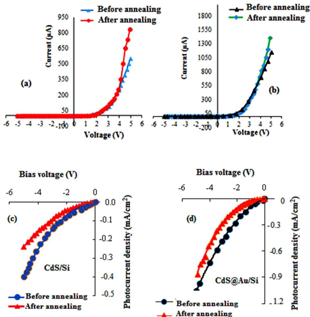
Fig. 6 (a) Dark  $I$ - $V$  characteristics of CdS/Si heterojunction before and after annealing, (b) dark  $I$ - $V$  characteristics of Au-decorated CdS/Si heterojunction before and after annealing, (c)  $I$ - $V$  characteristics of CdS/Si under illumination before and after annealing, and (d)  $I$ - $V$  characteristics of Au-decorated CdS/Si under illumination before and after annealing.
