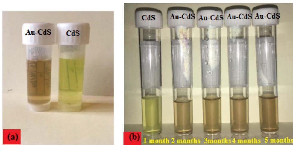
**Fig. 10** (a) Photograph of freshly prepared CdS and Au-decorated CdS colloids (b) photograph of colloids after five months of storage in the lab, and (c) variation of responsivity of CdS/Si and Au-decorated CdS/Si photodetectors with storage time.
