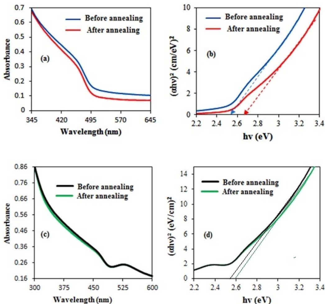
Fig. 4 (a) UV-vis absorption spectra of CdS films before and after annealing, (b)  $(\alpha h\nu)^2$  versus photon energy plot of CdS, (c) UV-vis absorption spectra of Au-decorated CdS films before and after annealing, and (d)  $(\alpha h\nu)^2$  against photon energy plot of Au-decorated CdS.
