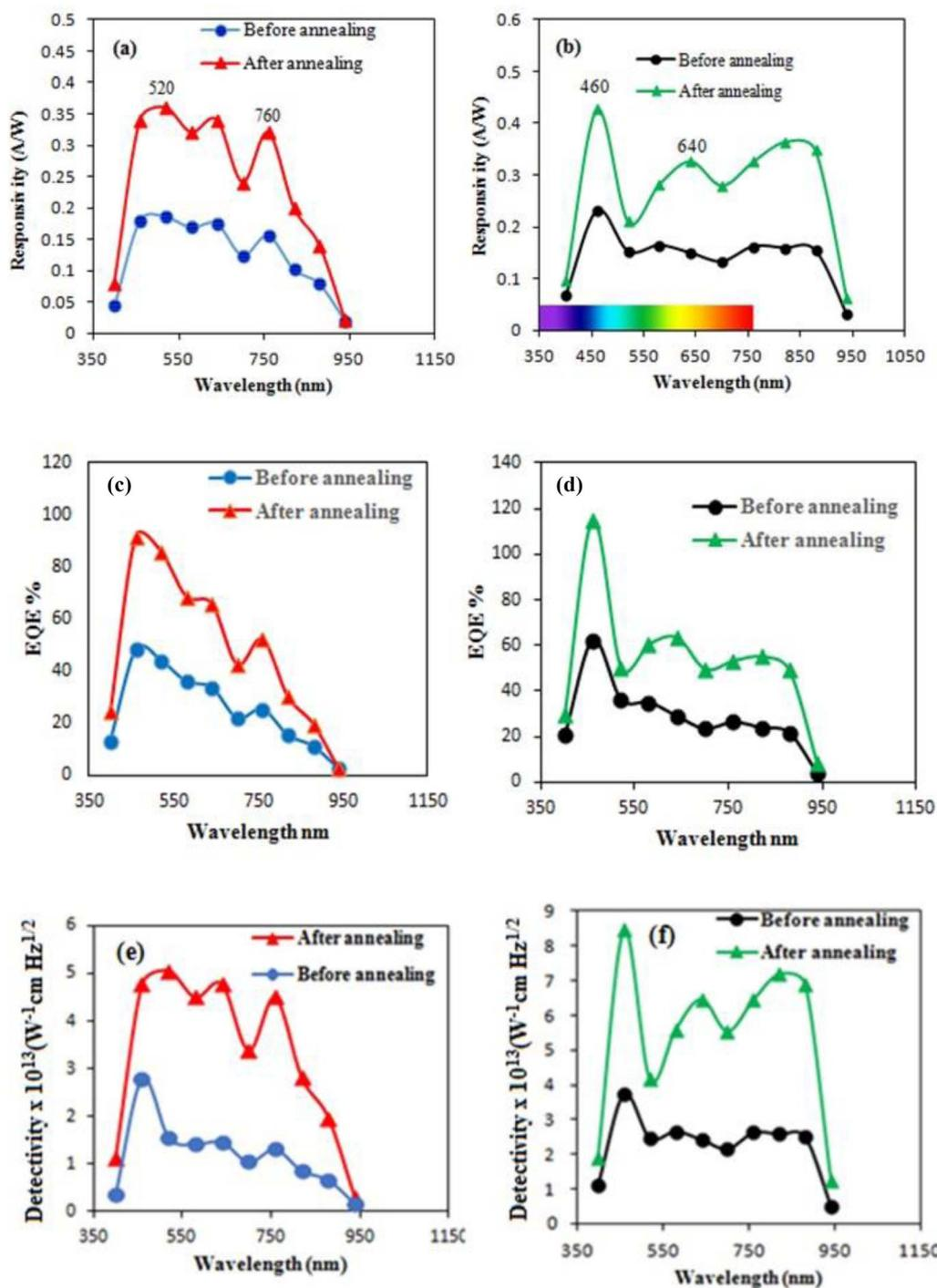
Fig. 9 (a) Responsivity of self-driven CdS/Si photodetector before and after annealing, (b) responsivity plot of Au-decorated CdS/Si photodetector, (c) EQE of CdS/Si photodetector, (d) EQE of Au-decorated CdS/Si (e) detectivity of CdS/Si photodetector, and (f) detectivity of Au-decorated CdS/Si heterojunction after annealing.
