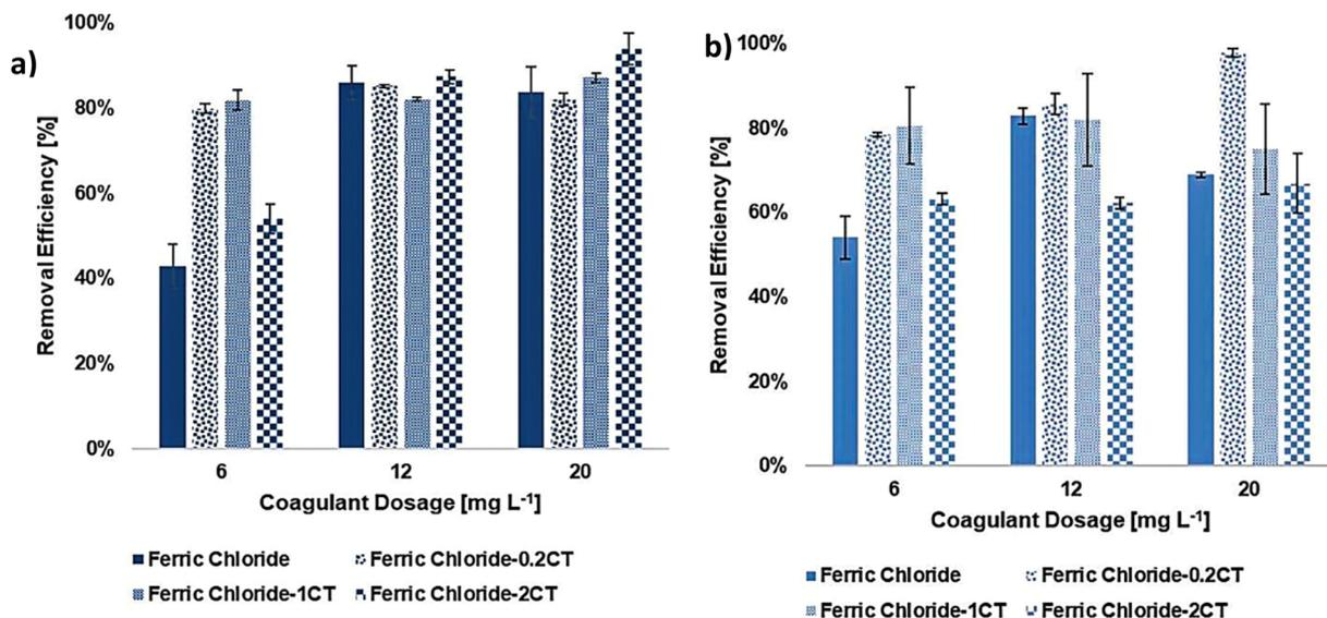
Fig. 7 Removal efficiency of (a) PS, and (b) PE under different  $\text{FeCl}_3$ -CT dosages. Initial pH 7, initial concentration of  $300 \text{ mg L}^{-1}$ , adapted with permission from ref. 26, Copyright, Elsevier, 2025.
